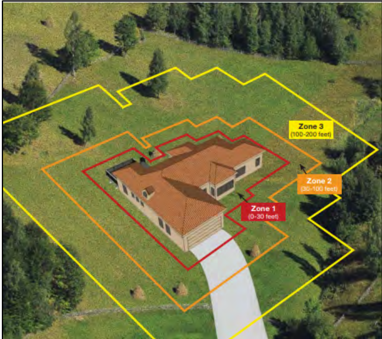
Figure 4.4. Defensible space zones providing clearance between a structure and adjacent woodland or forest fuels.
