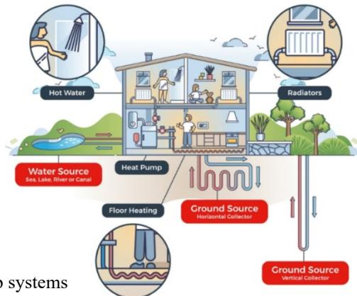
Geothermal Ground-Coupled Heat Pump systems
