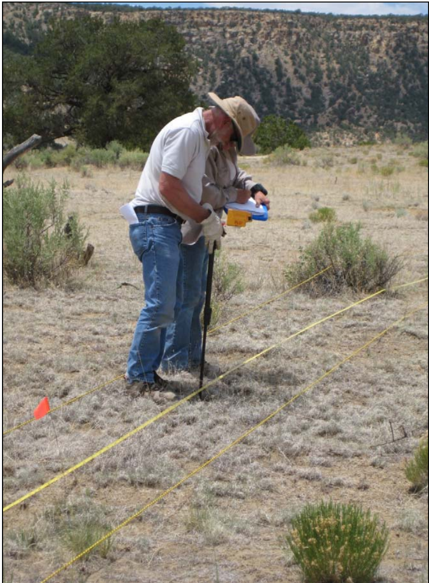
Figure 1. Using an optical laser device to measure cover along a 50-m long transect line.
