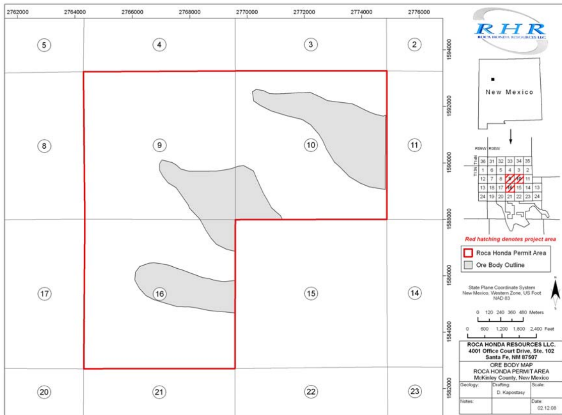
Figure 7-6. Uranium Ore Body at the Roca Honda Permit Area
