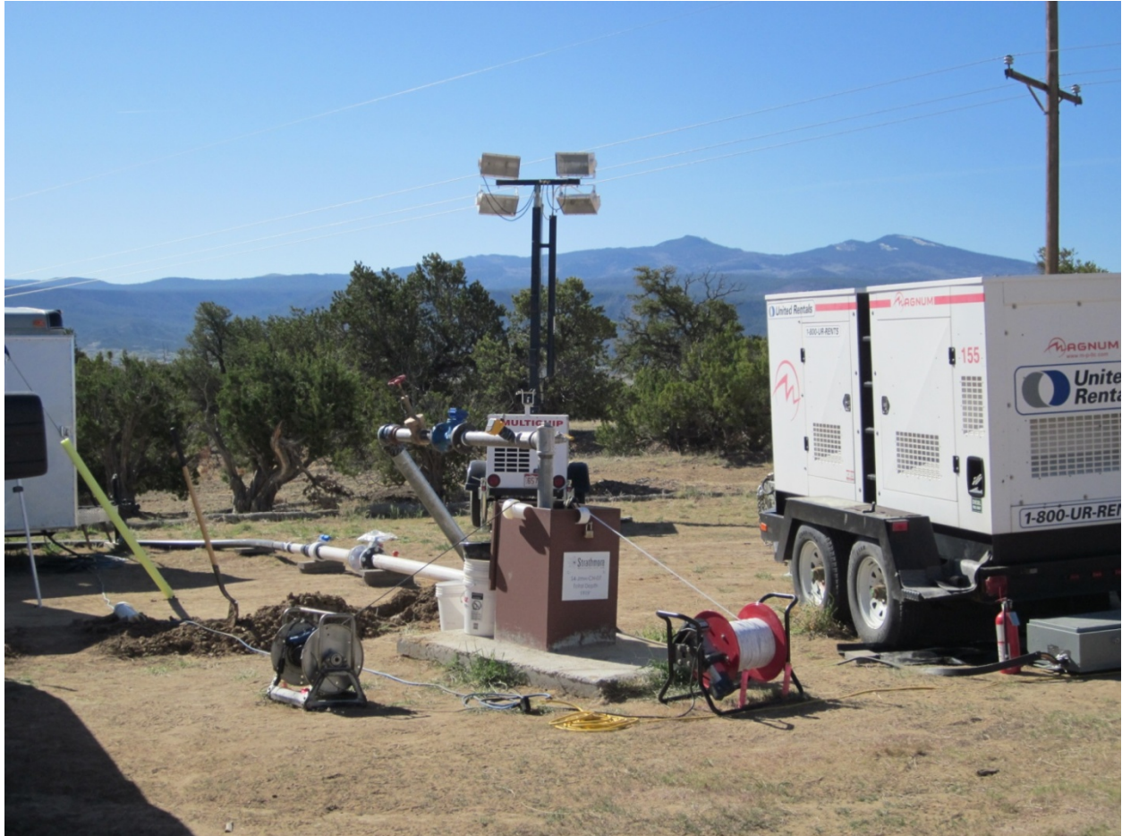
Figure 8. RHR Pumping Well S-4 during Aquifer Test
