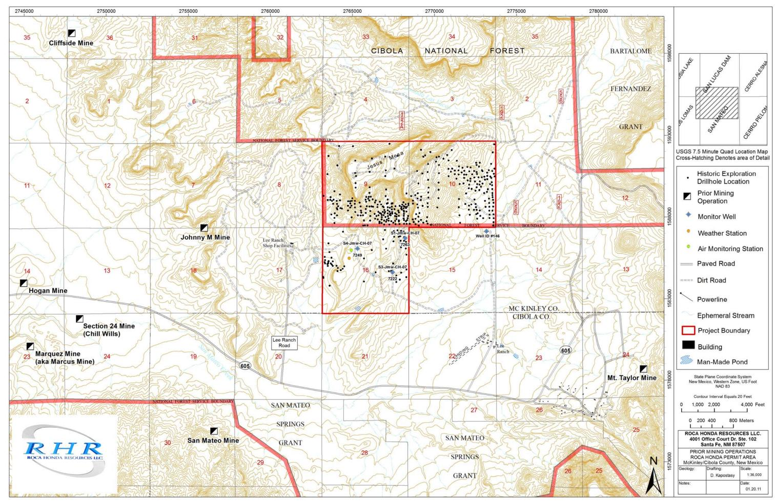
Figure 10-1. Topographic Base Map Showing Prior Mining Operations (1:36,000)
