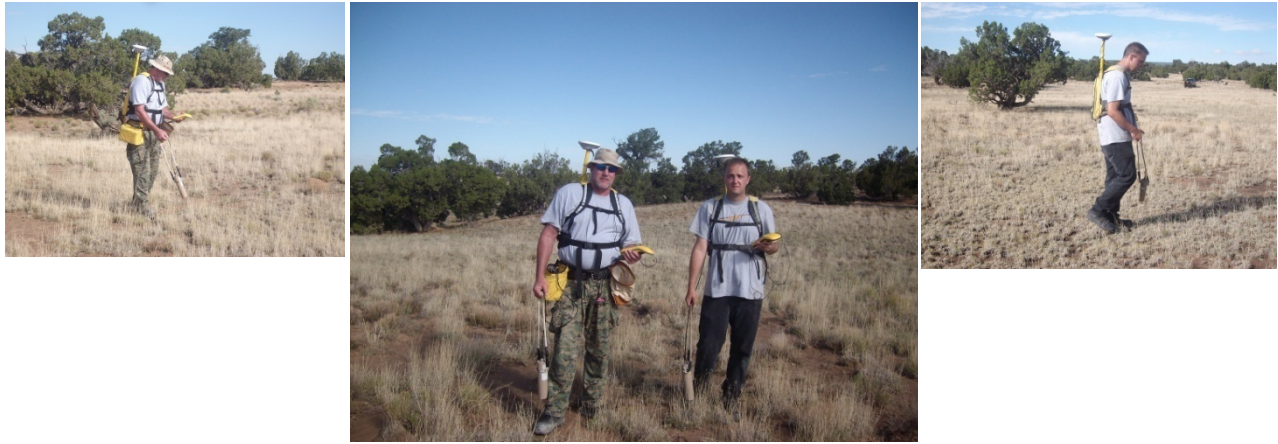
Scott Kaplan and Justin Ebright, conducting walkover gamma scanning in Section 16 of the Roca Honda Site using 2x2 inch NaI detectors with Trimble GPS units, July 2010.
