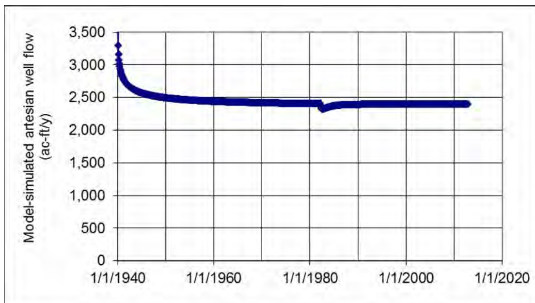
Figure 6.28. Simulated artesian well discharge.
