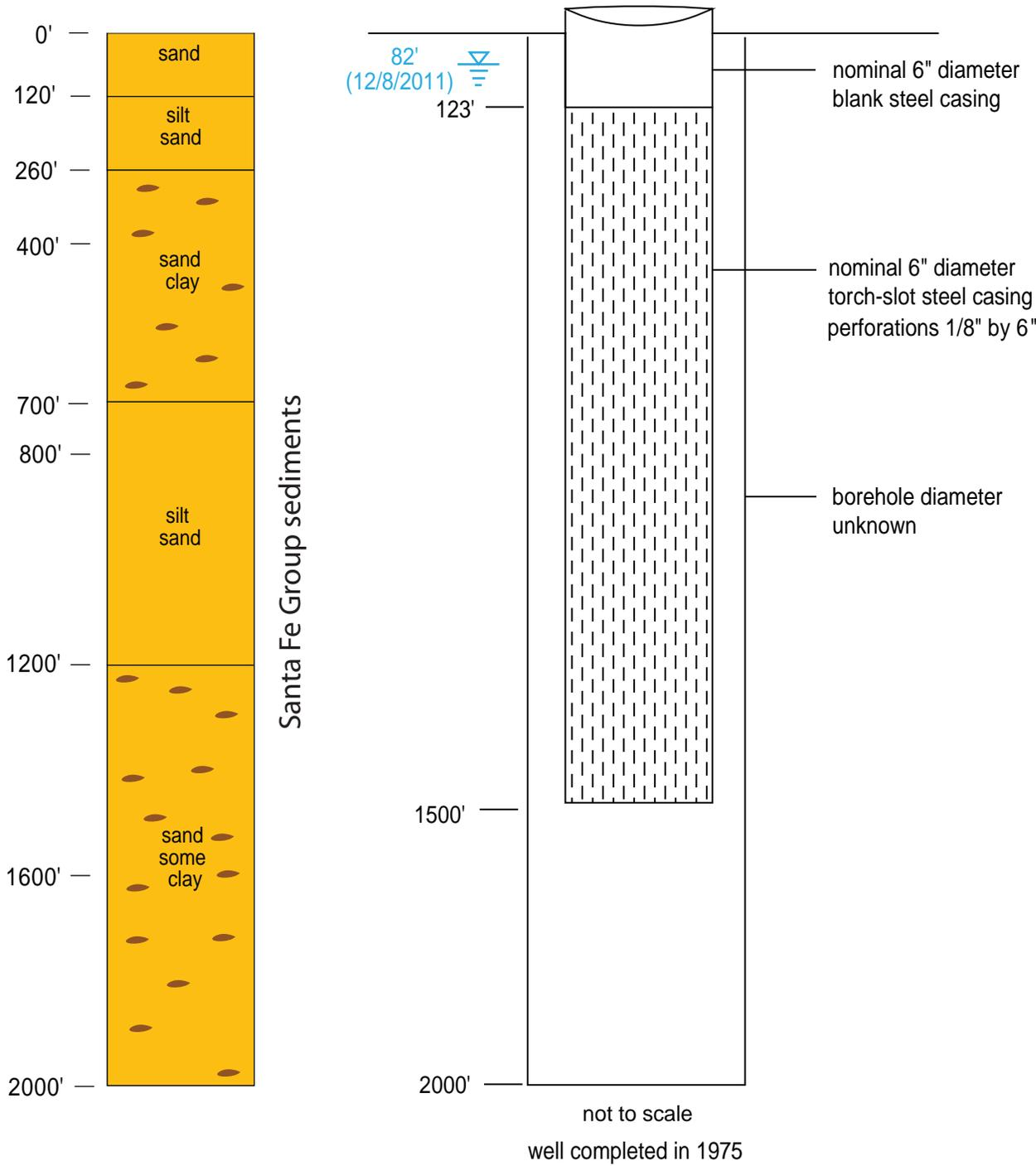
Figure B14. Well completion diagram for LRG-4652-S-13 (MW-4), Copper Flat Mine, Sierra County, New Mexico.
