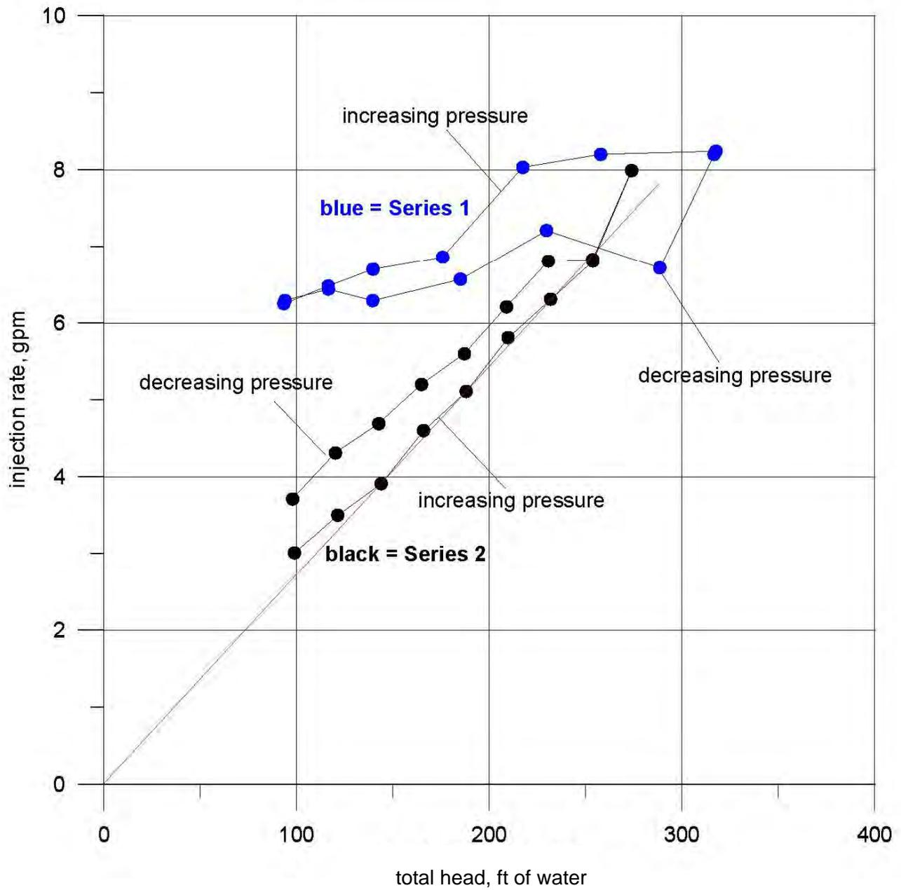
Figure 6. Pressure injection test, New Mexico Copper GWQ 11-24, Zone 2 (150-197 ft), Series 1 and 2, July 30, 2011.
