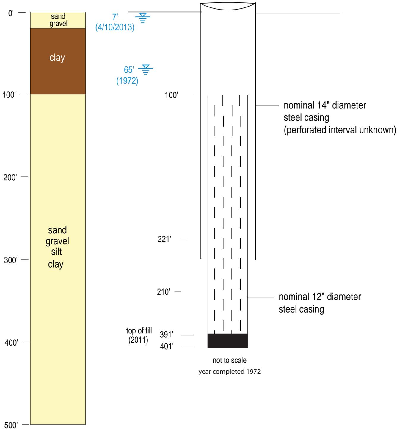
Figure B11. Well completion diagram for LRG-4652-S-10 (GWQ-1, North Inspiration, Well IDW-2, S-10), Copper Flat Mine, Sierra County, New Mexico.
