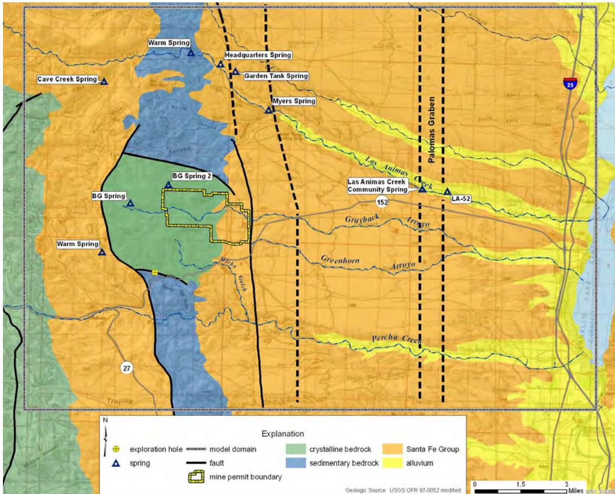
Figure 4.4. Hydrogeologic units and mapped spring locations.
