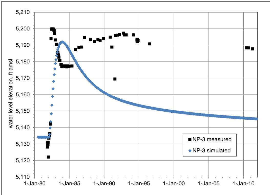
Figure 6.24. Measured and simulated water-level hydrographs in NP-3.
