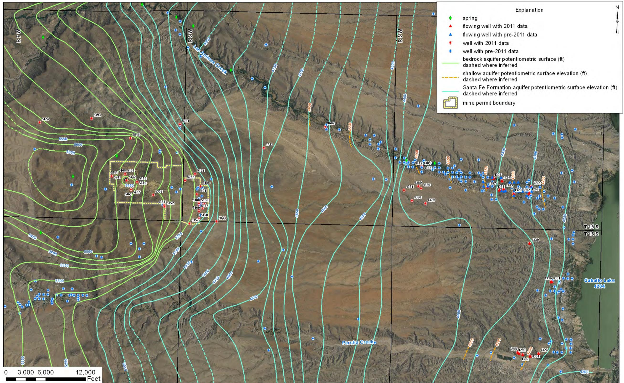
Figure 5.1. Regional water-level measurements and potentiometric surface contours.
