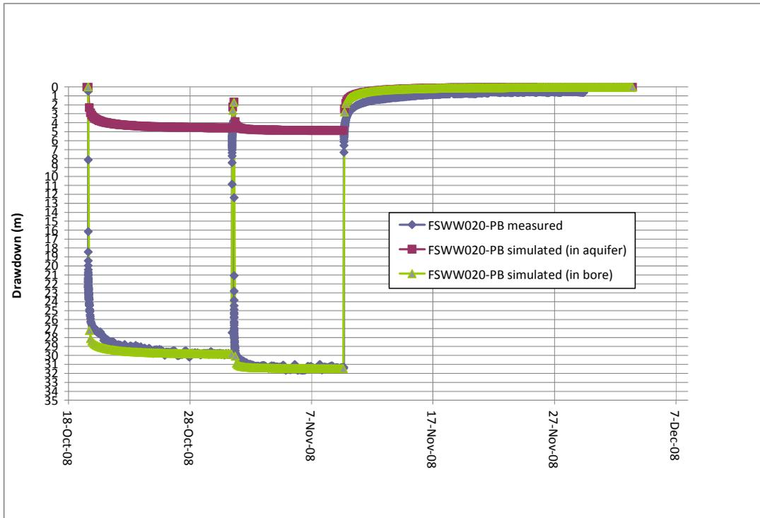
Figure 5.6. Measured and simulated aquifer test drawdown, FSWW020-PB.
