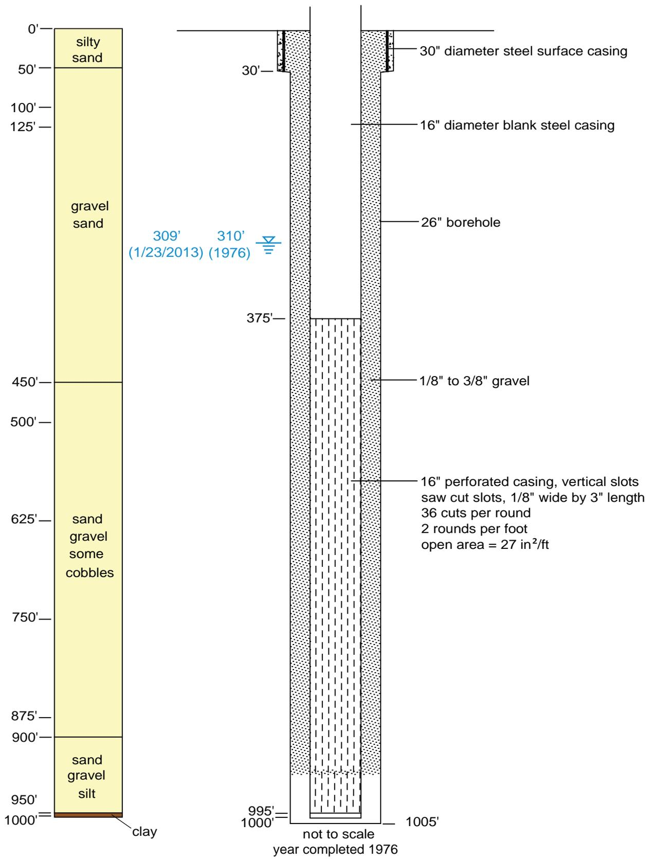
Figure B2. Well completion diagram for LRG-4652-S (PW-2),
