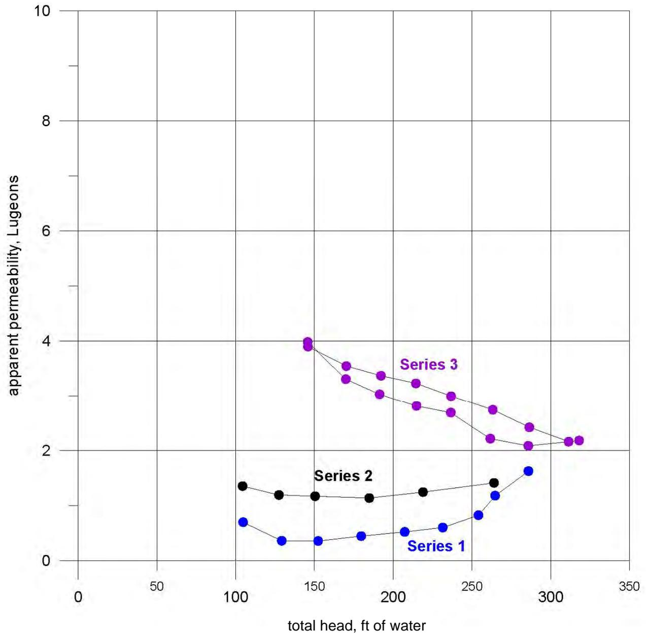
Figure 5. Apparent permeability from pressure injection tests, New Mexico Copper GWQ 11-24, Zone 1 (100-147 ft), Series 1 and 2 (centrifugal pump), and Series 3 (positive displacement pump), July 27, 2011.
