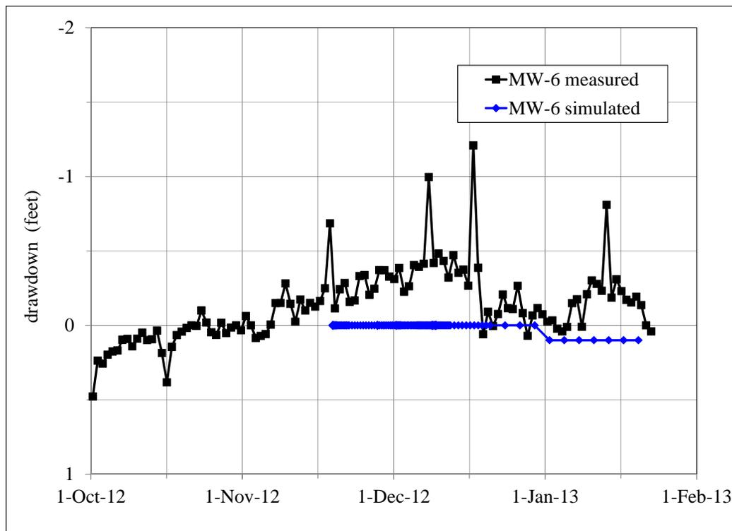
Figure 6.39. Measured and simulated water-level hydrographs in MW-6.
