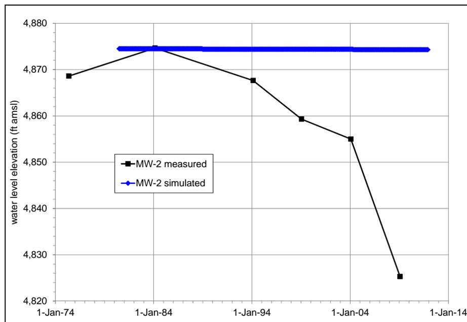
Figure 6.20. Measured and simulated water-level hydrographs in MW-2.
