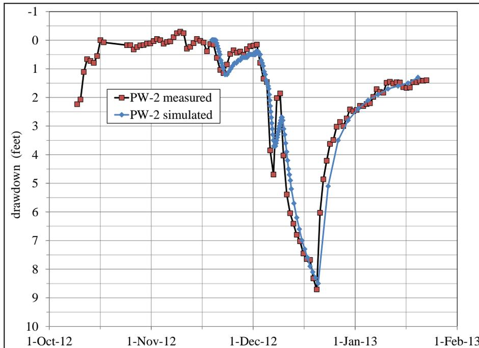
Figure 6.33. Measured and simulated water-level hydrographs in PW-2.
