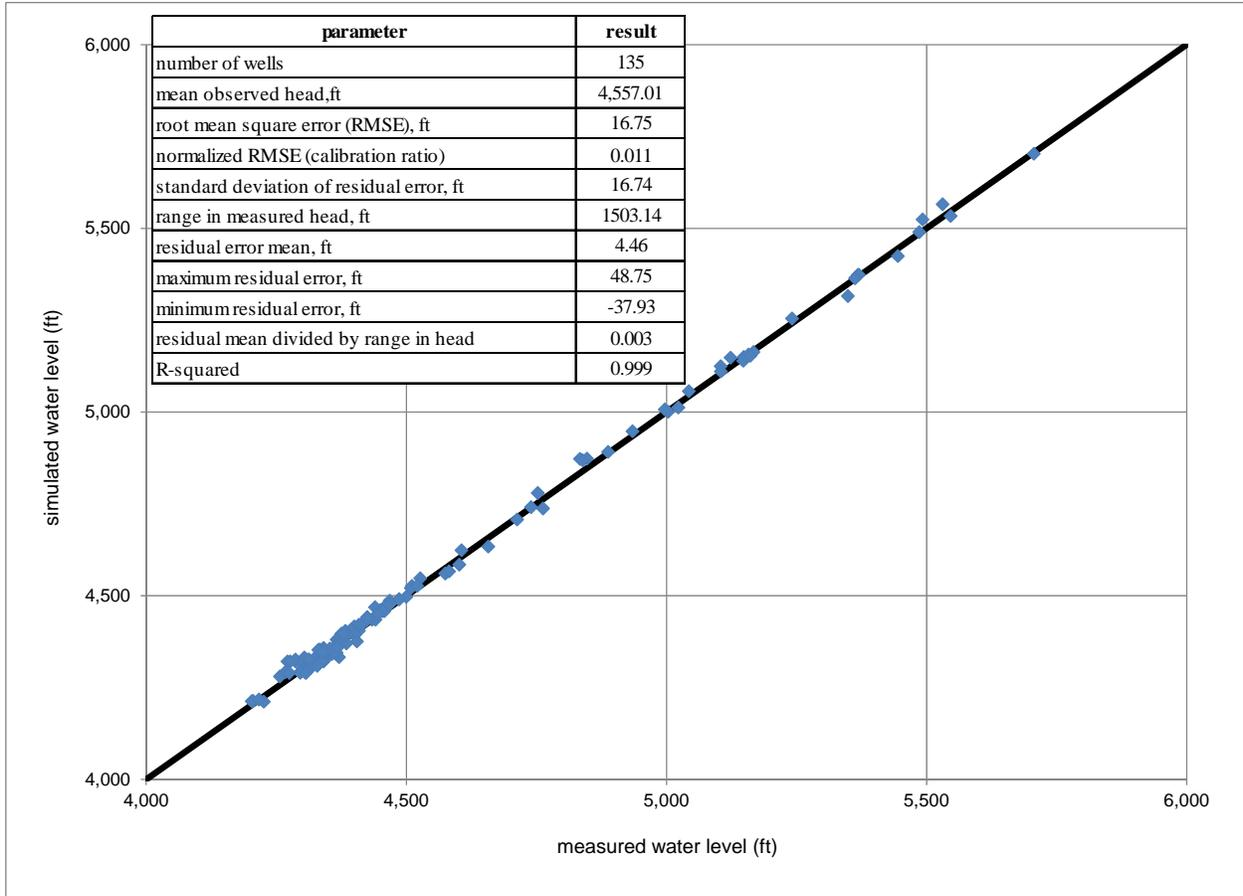
Figure 6.10. Comparison of measured and simulated water levels.
