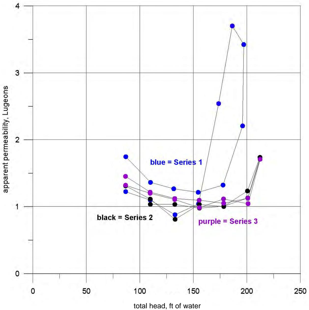
Figure 13. Apparent permeability from pressure injection test, New Mexico Copper GWQ 11-25, Zone 3 (207-251 ft), Series 1, 2, and 3, August 24, 2011.
