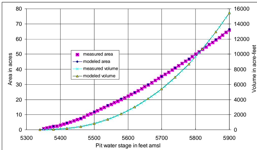
Figure 2.2. Measured and modeled pit stage-area-volume.
