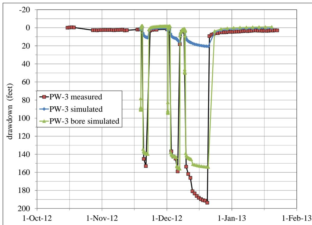
Figure 6.32. Measured and simulated water-level hydrographs in PW-3.
