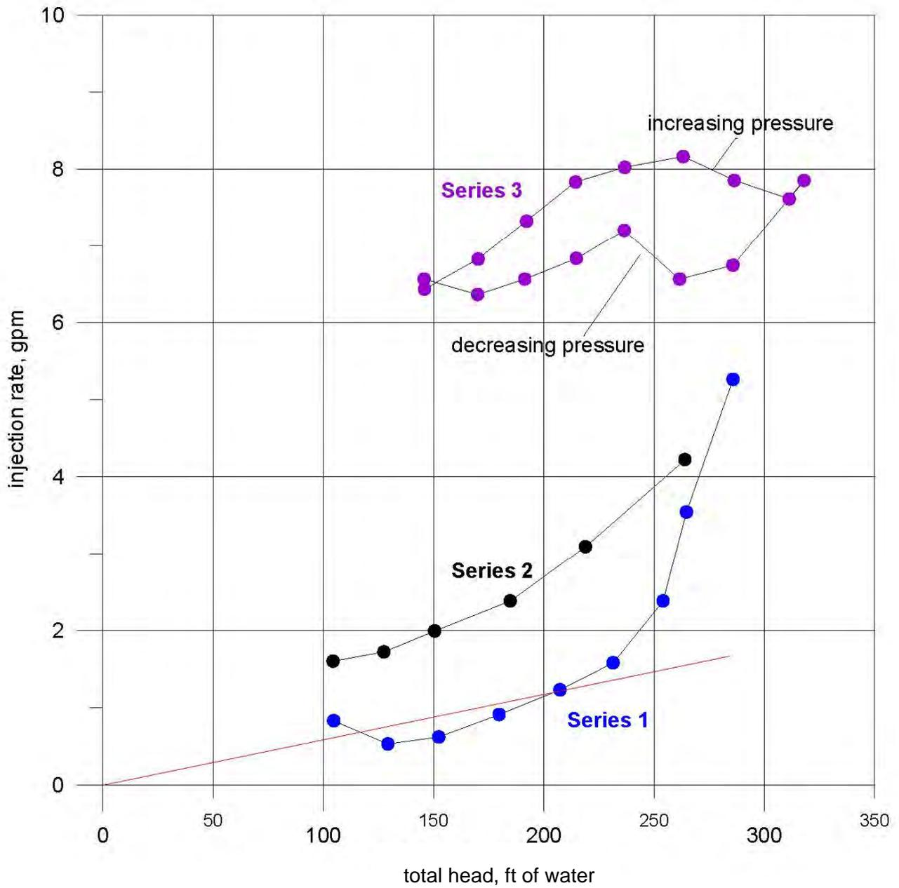
Figure 4. Pressure injection tests, New Mexico Copper GWQ 11-24, Zone 1 (100-147 ft), Series 1 and 2 (centrifugal pump), and Series 3 (positive displacement pump), July 27, 2011.
