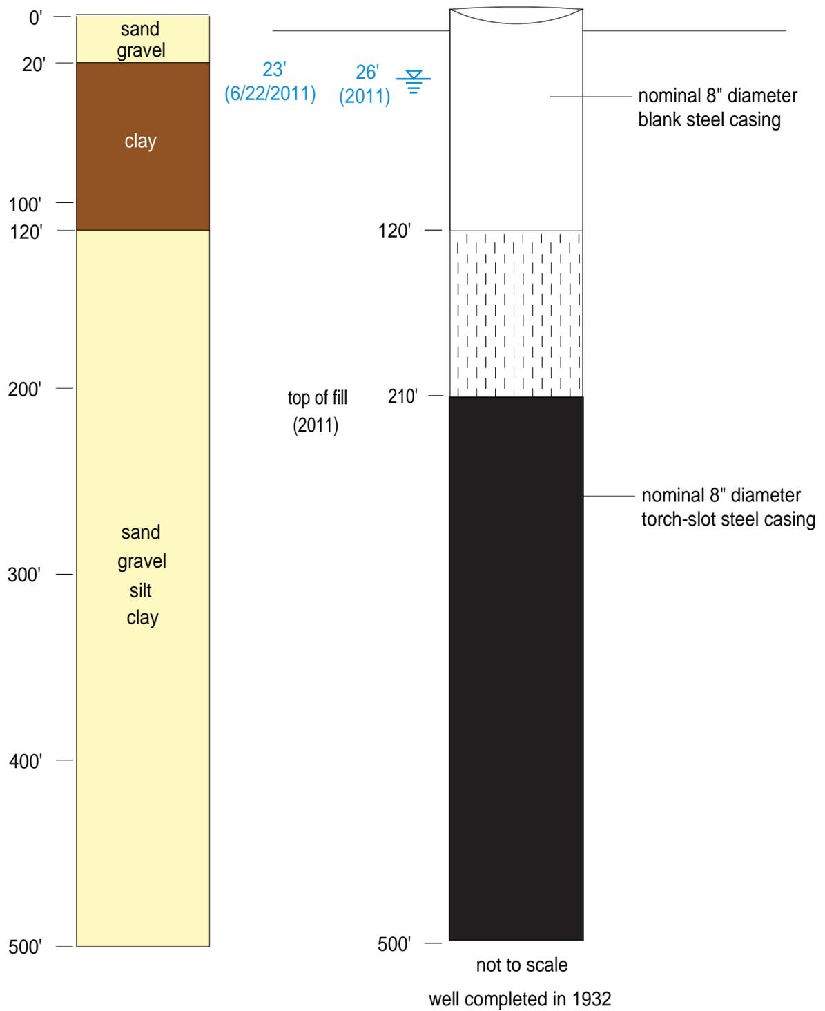
Figure B8. Well completion diagram for LRG-4652-S-7 (Irwin Well), Copper Flat Mine, Sierra County, New Mexico.
