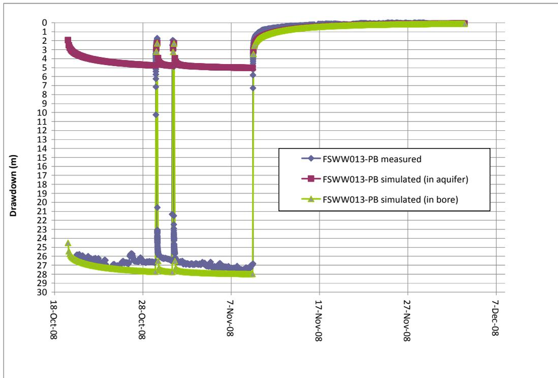
Figure 5.3. Measured and simulated aquifer test drawdown, FSWW013-PB.
