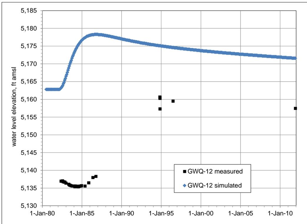
Figure 6.27. Measured and simulated water-level hydrographs in GWQ-12.
