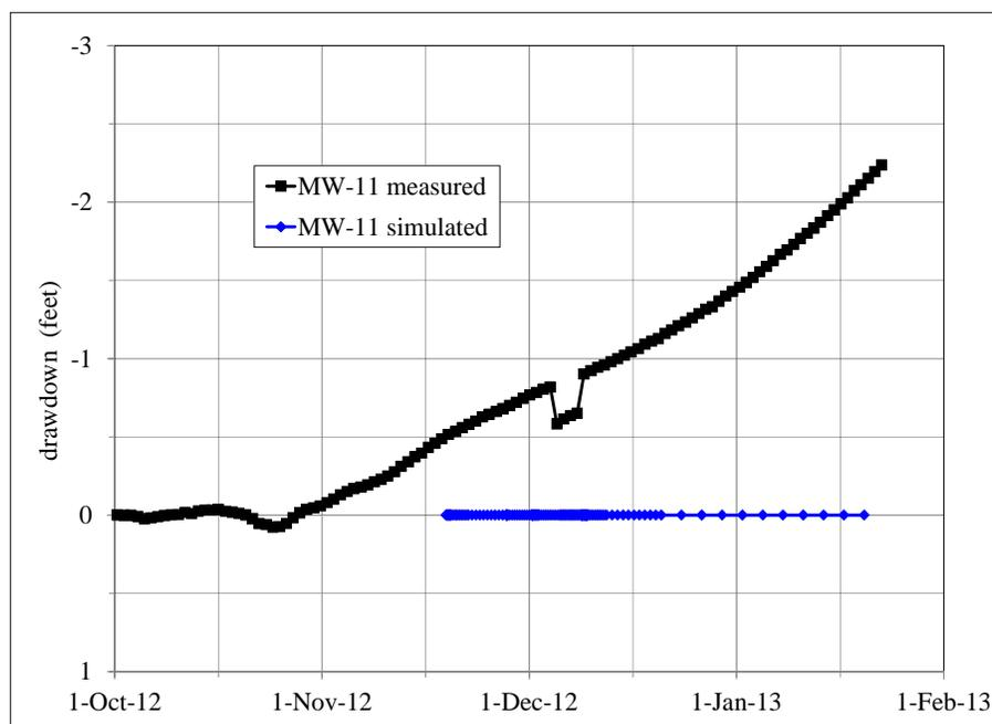
Figure 6.37. Measured and simulated water-level hydrographs in MW-11.
