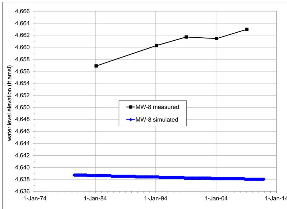
Figure 6.21. Measured and simulated water-level hydrographs in MW-8.
