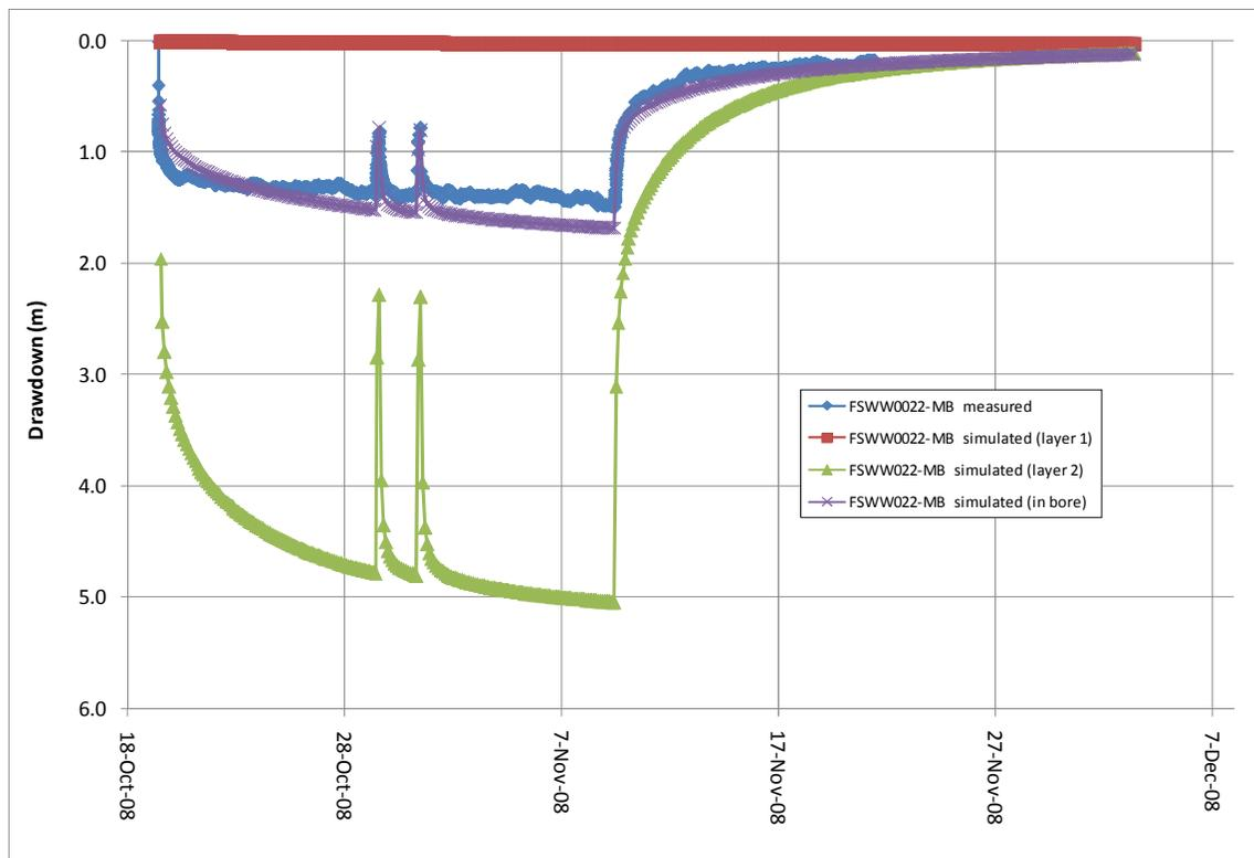
Figure 5.5. Measured and simulated aquifer test drawdown, FSWW022-MB.
