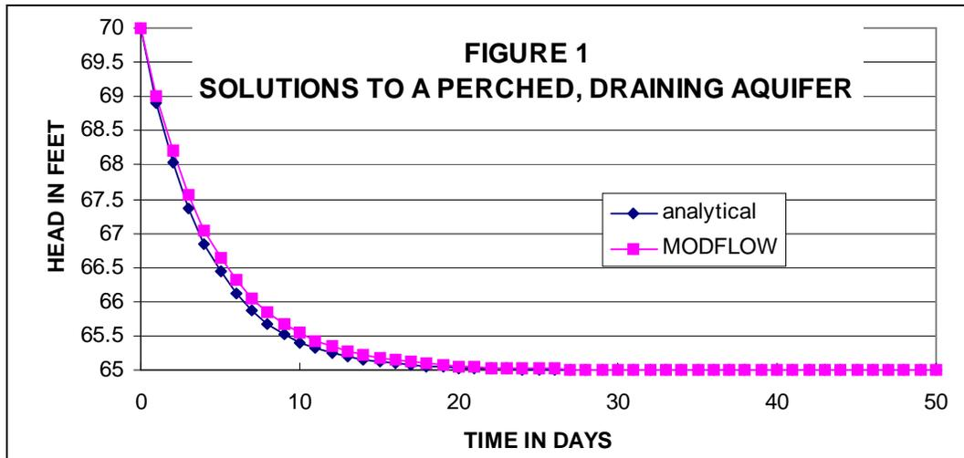
Figure 1 shows that the isolated layer drains as expected, with a reasonable match of the analytical solution. Furthermore, a 1-point implicit finite difference spreadsheet solution exactly matched the MODFLOW solution. Inspection of the mass balance table in the simulation output also shows that the water from Layer 1 enters aquifer storage or exits through constant heads in the active Layers 10-14.
