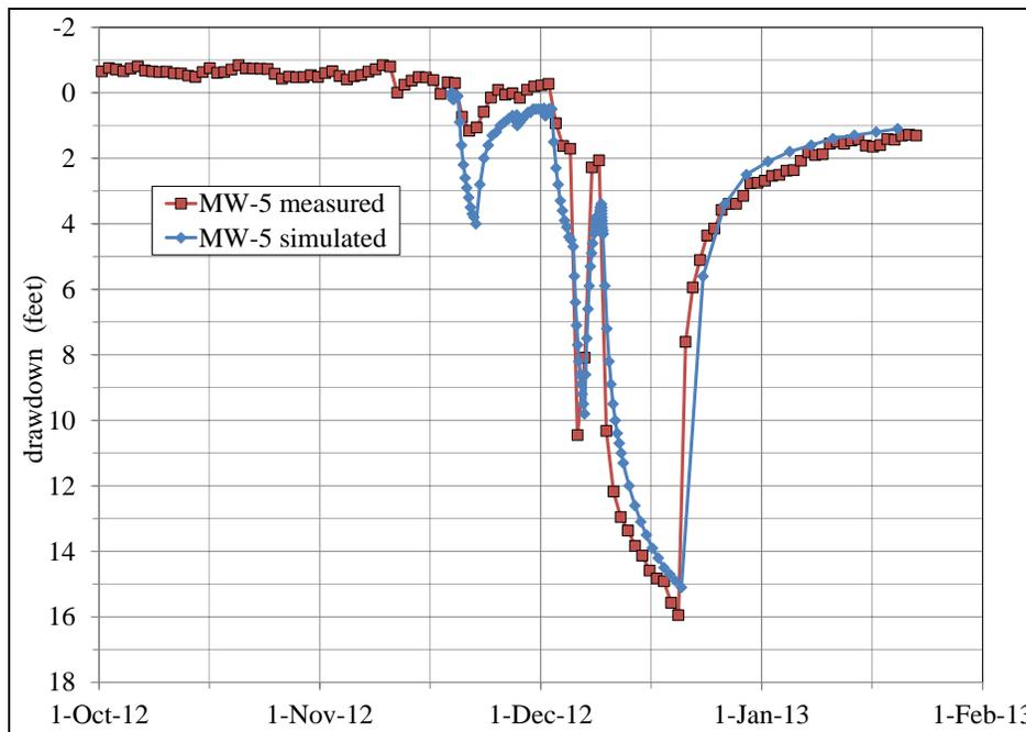
Figure 6.35. Measured and simulated water-level hydrographs in MW-5.
