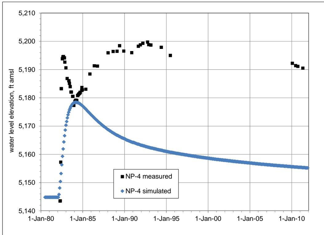
Figure 6.25. Measured and simulated water-level hydrographs in NP-4.
