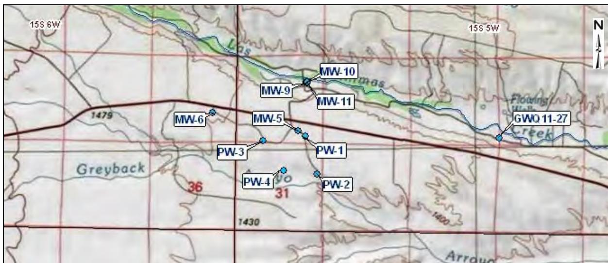
Figure 5.15. Aquifer test pumping and observation wells.
