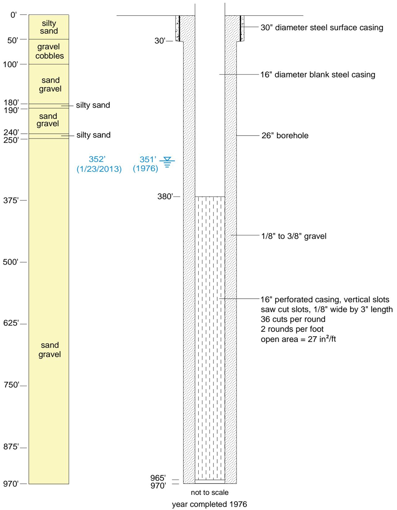
Figure B3. Well completion diagram for LRG-4652-S-2 (PW-3),
