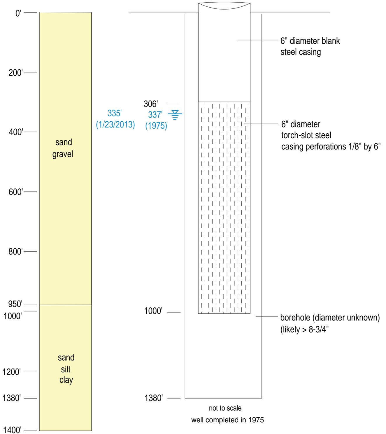
Figure B15. Well completion diagram for LRG-4652-S-14 (MW-5),
