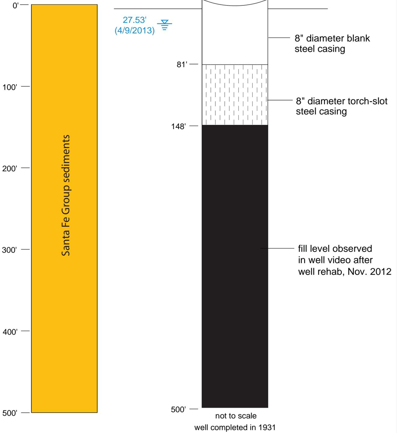
Figure B5. Well completion diagram for LRG-4652-S-4 (GWQ-8), Copper Flat Mine, Sierra County, New Mexico.
