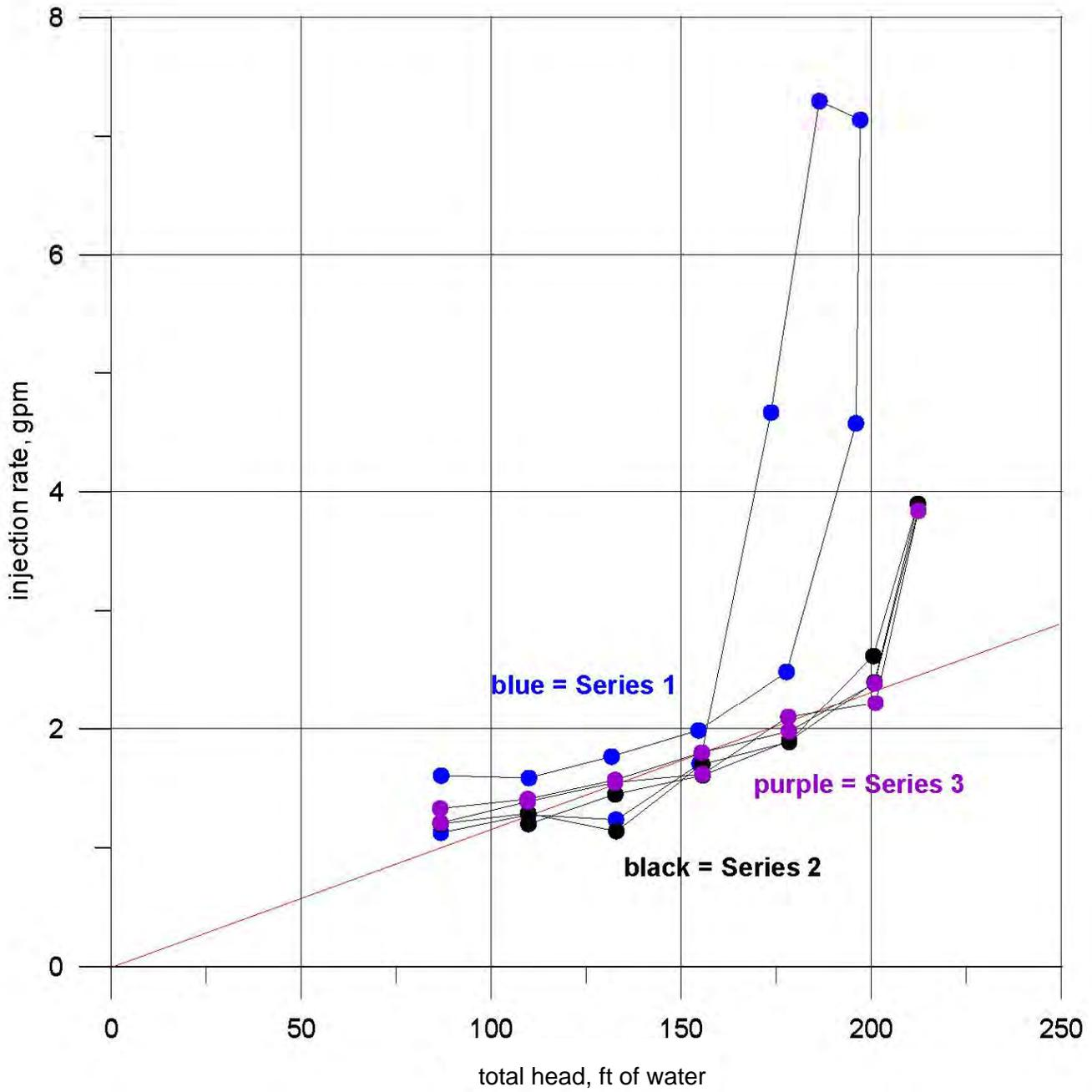
Figure 12. Pressure injection test, New Mexico Copper GWQ 11-25, Zone 3 (207-251 ft), Series 1, 2 and 3, August 24, 2011.
