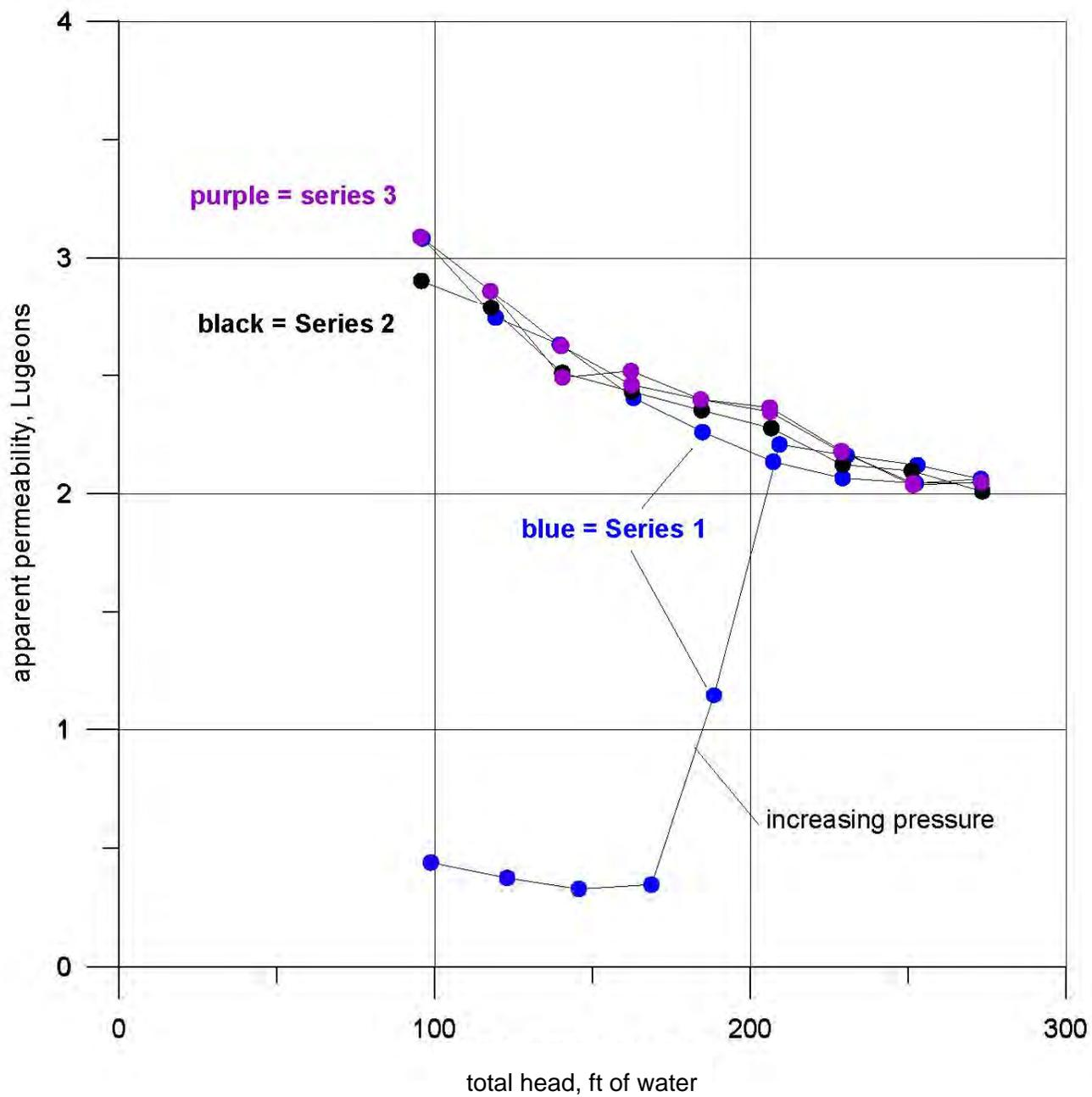
Figure 9. Apparent permeability from pressure injection test, New Mexico Copper GWQ 11-24, Zone 3 (204-251 ft), Series 1, 2, and 3, August 1, 2011.
