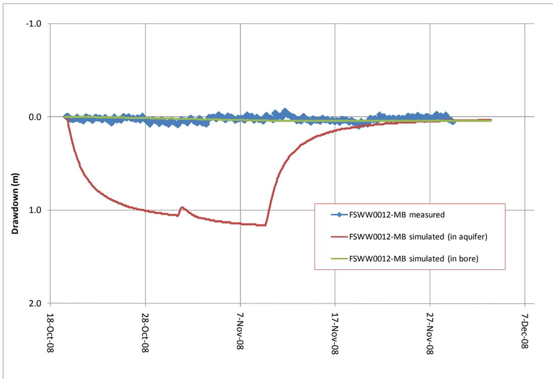
Figure 5.8. Measured and simulated aquifer test drawdown, FSWW012-MB.
