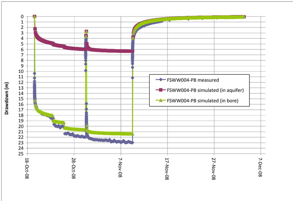
Figure 5.1. Measured and simulated aquifer test drawdown, FSWW004-PB.
