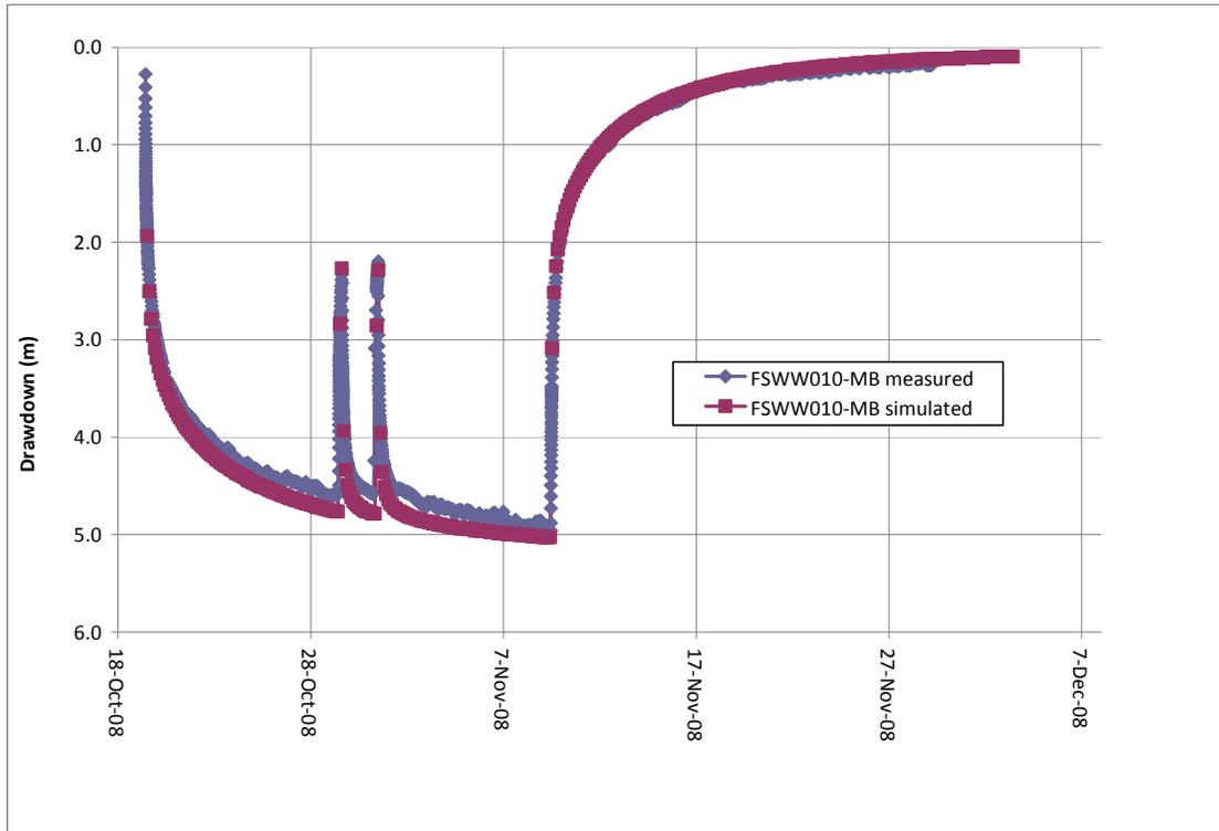
Figure 5.4. Measured and simulated aquifer test drawdown, FSWW010-MB.
