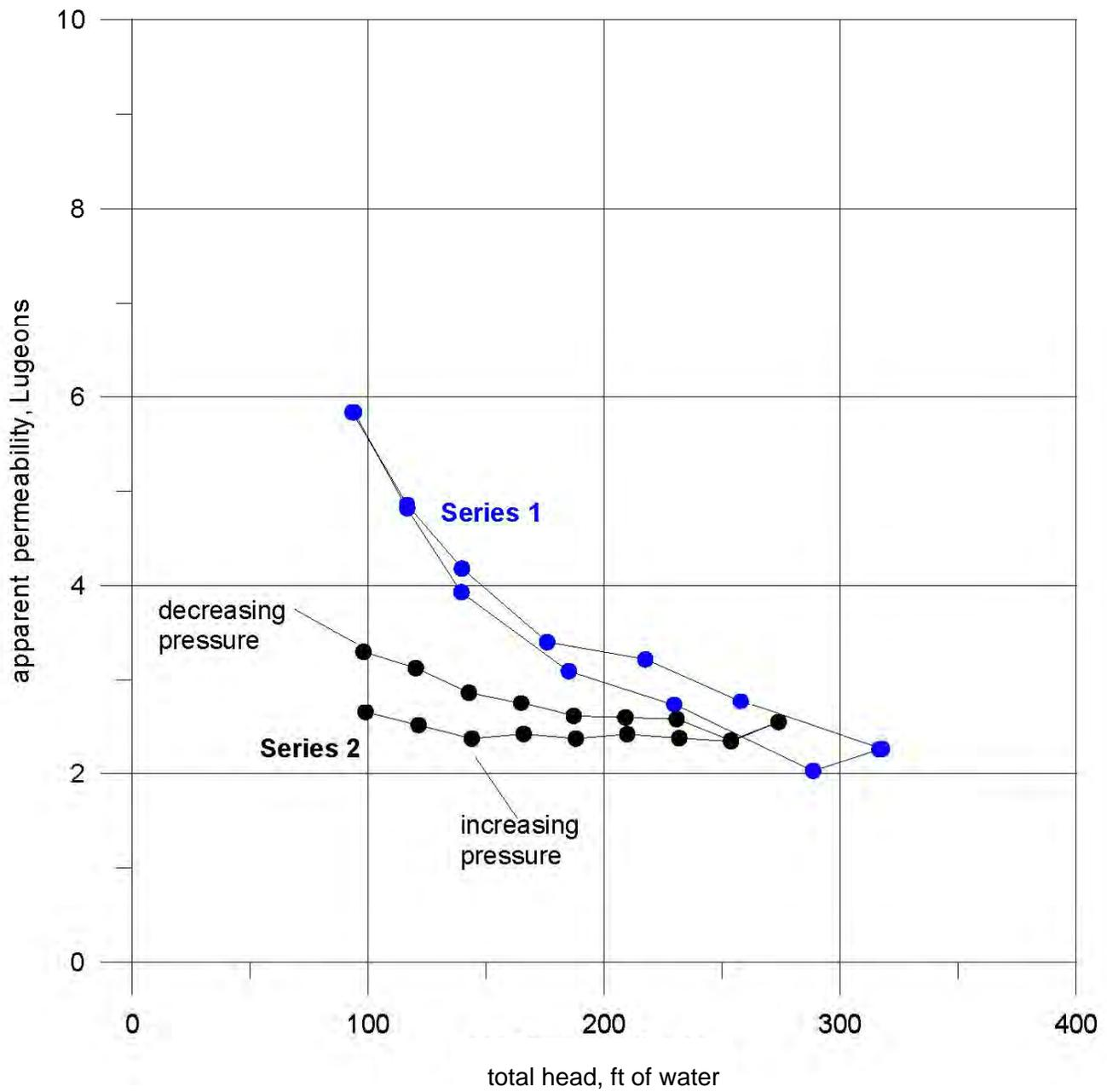
Figure 7. Apparent permeability from pressure injection test, New Mexico Copper GWQ 11-24, Zone 2 (150-197 ft), Series 1 and 2, July 30, 2011.
