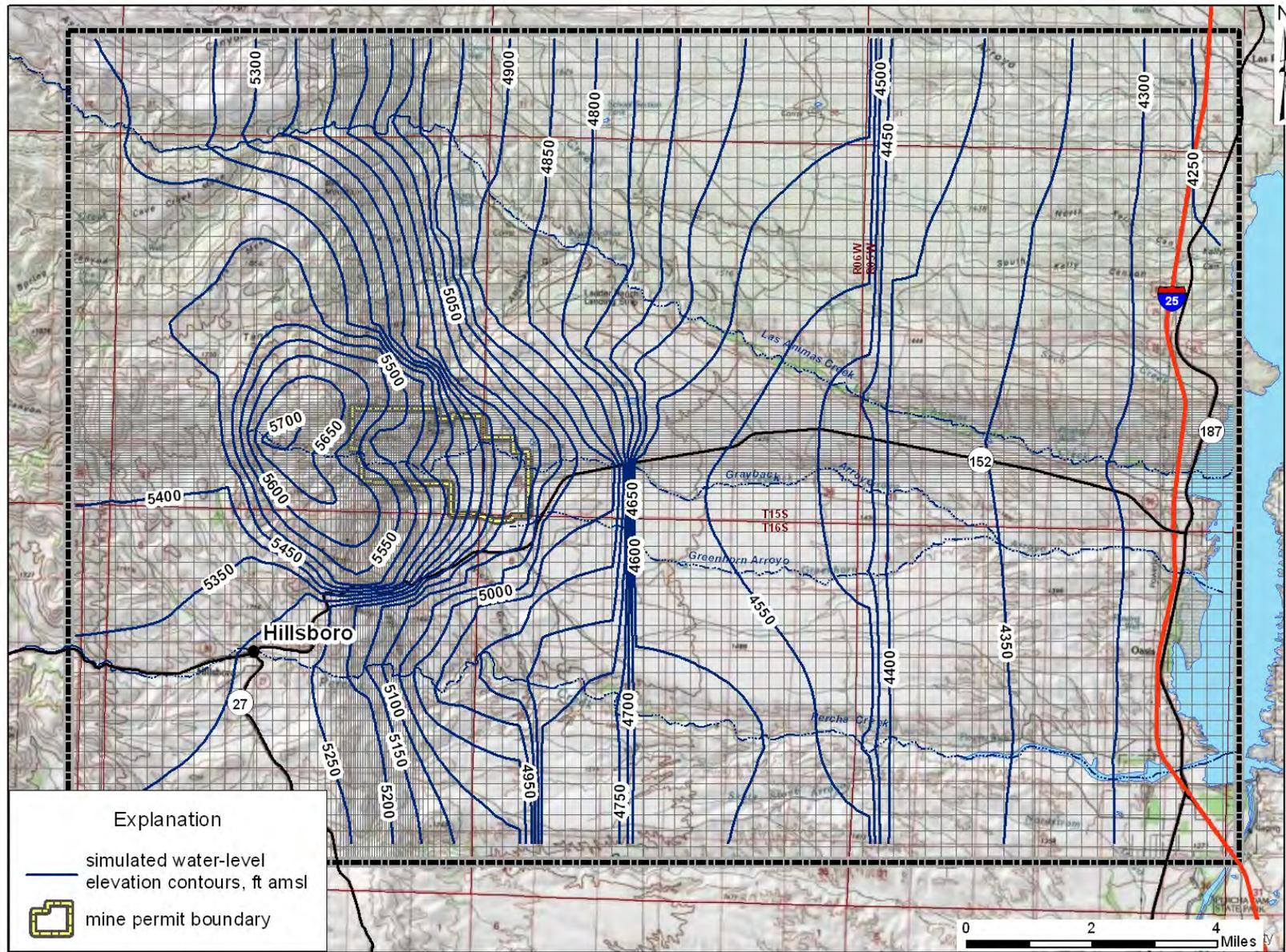
Figure 6.11. Contours of simulated 2012 groundwater levels.
