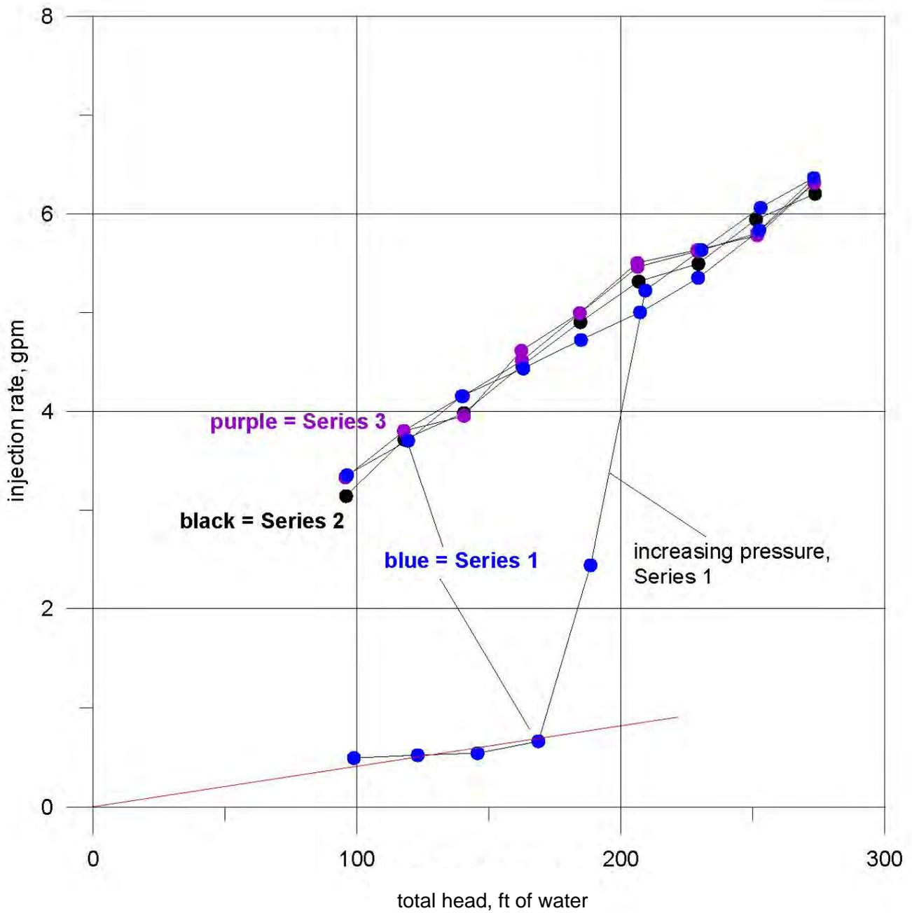
Figure 8. Pressure injection test, New Mexico Copper GWQ 11-24, Zone 3 (204-251 ft), Series 1, 2, and 3, August 1, 2011.
