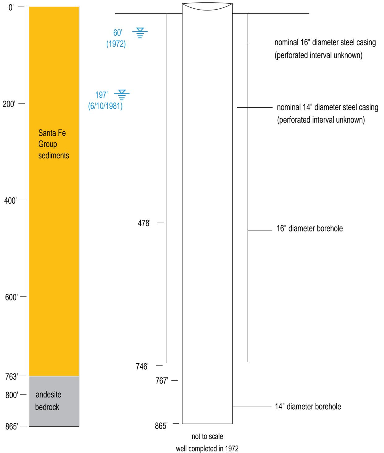
Figure B10. Well completion diagram for LRG-4652-S-9 (GWQ-9, South Inspiration, Well IDW-1), Copper Flat Mine, Sierra County, New Mexico.
