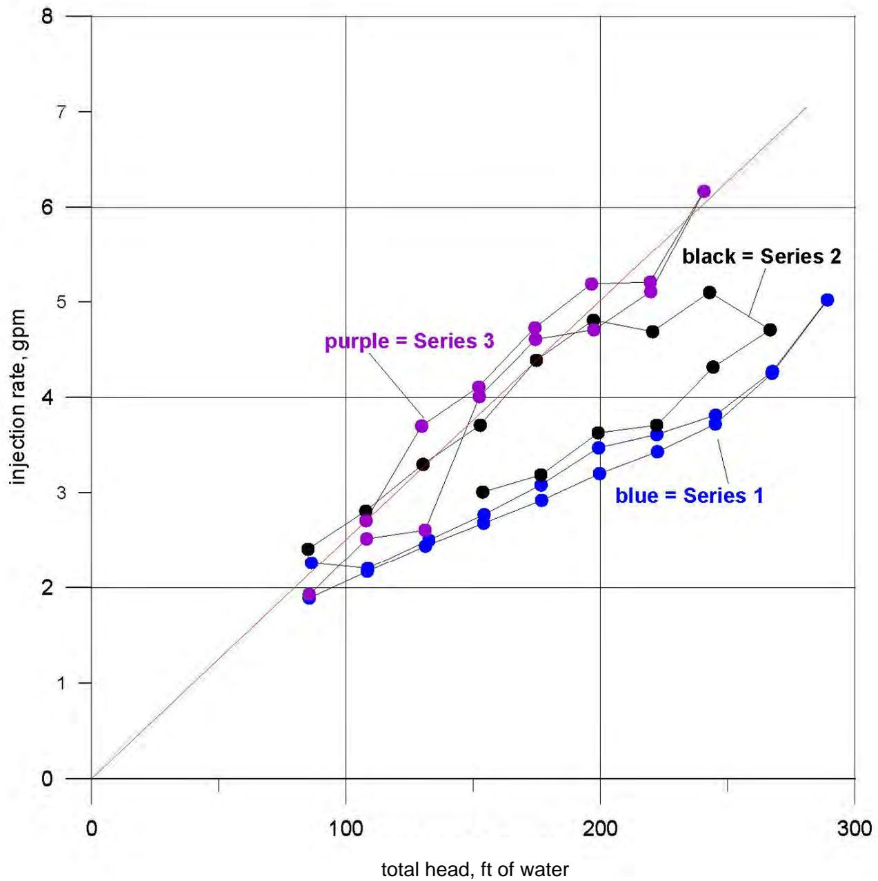
Figure 10. Pressure injection test, New Mexico Copper GWQ 11-25, Zone 2 (150-197.7 ft), Series 1, 2, and 3, August 16, 2011.
