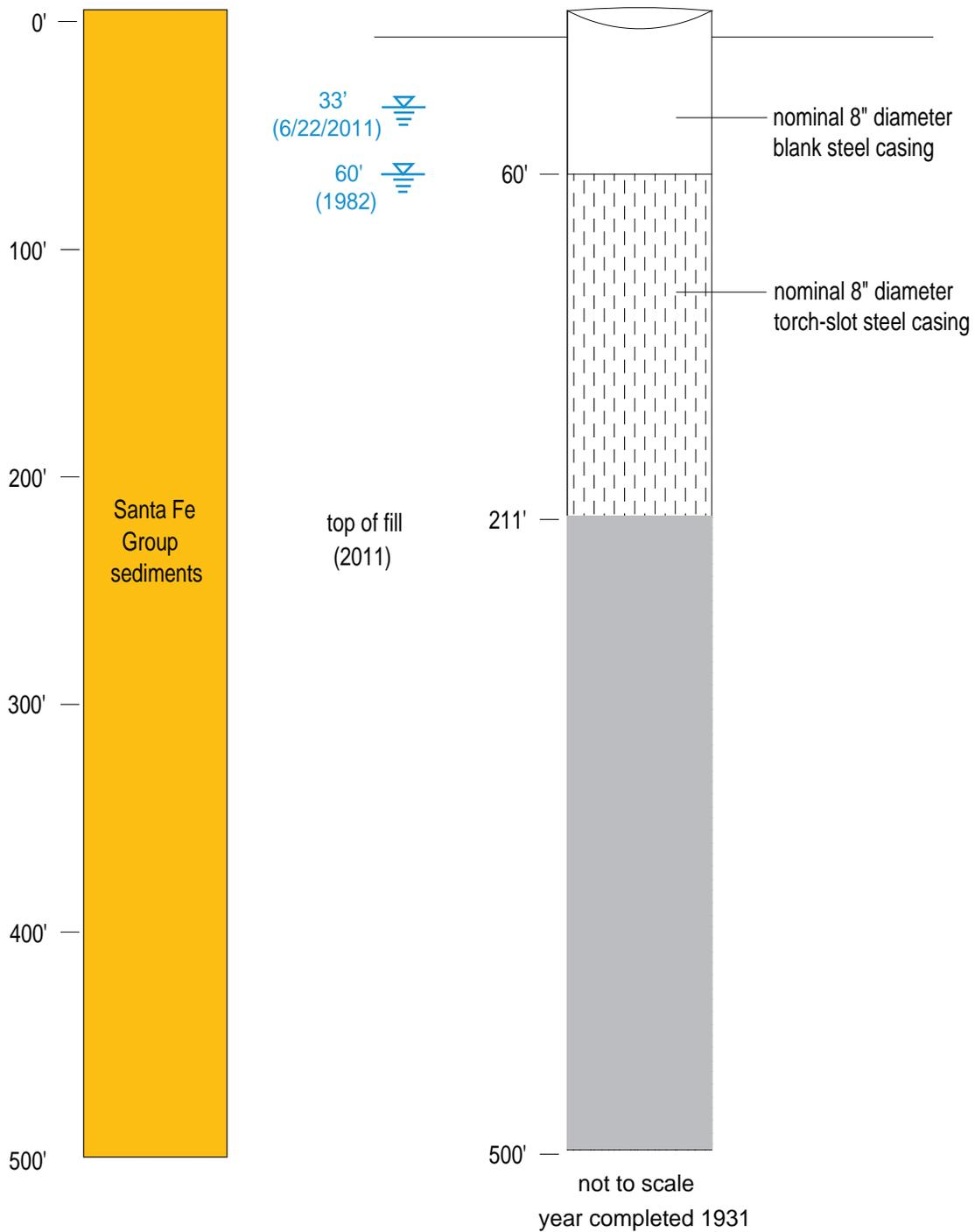
Figure B7. Well completion diagram for LRG-4652-S-6 (GWQ-2),
