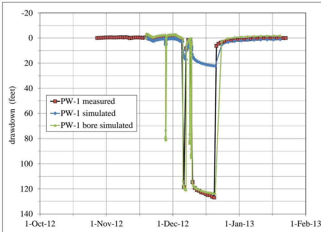
Figure 6.31. Measured and simulated water-level hydrographs in PW-1.
