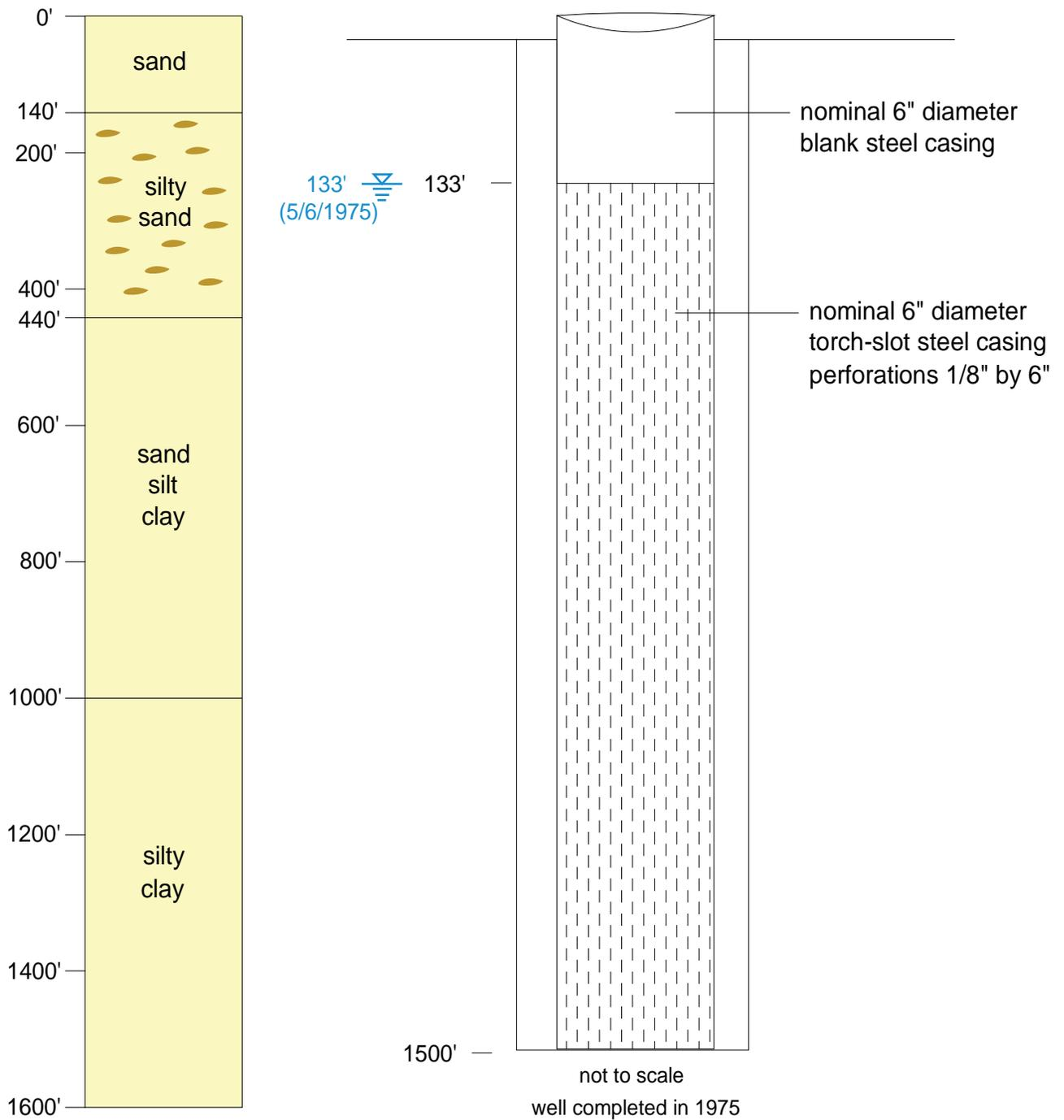
Figure B13. Well completion diagram for LRG-4652-S-12 (MW-2), Copper Flat Mine, Sierra County, New Mexico.
