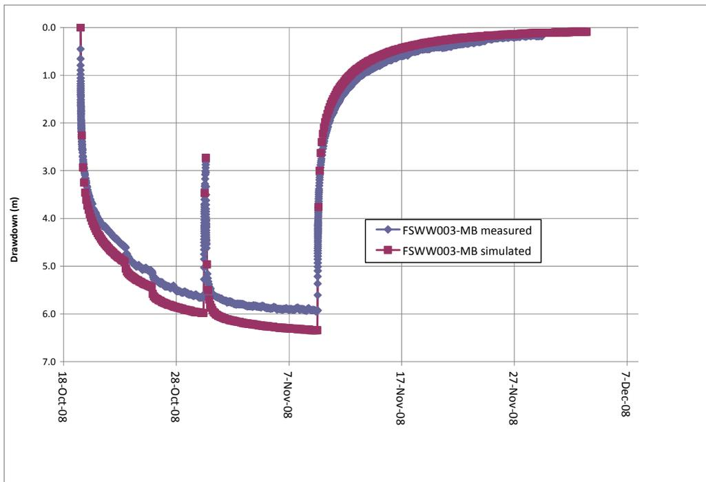
Figure 5.2. Measured and simulated aquifer test drawdown, FSWW003-MB.
