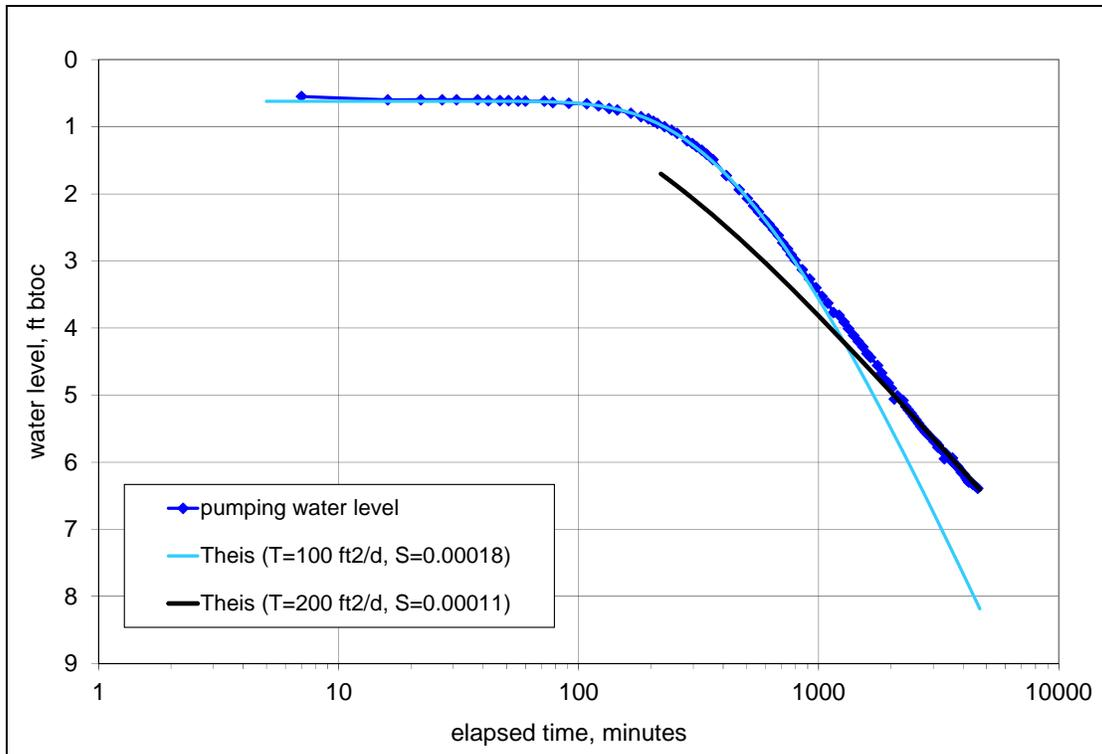
Figure 5.19. Drawdown in GWQ-15 during 1994 GWQ-17 pumping test.
