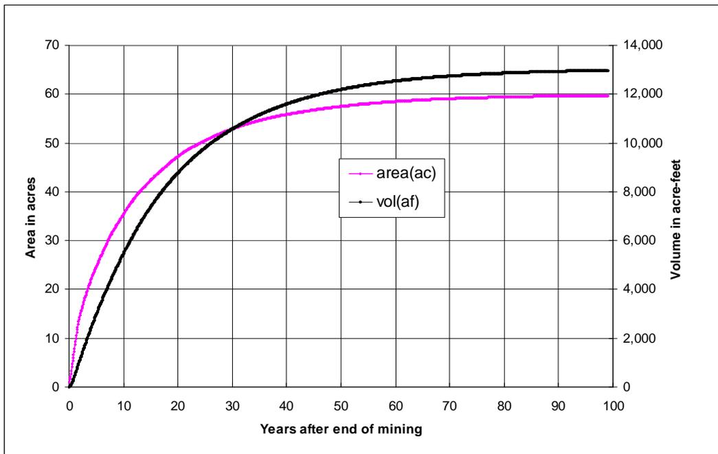
Figure 2.4. Projected pit water surface area and volume.
