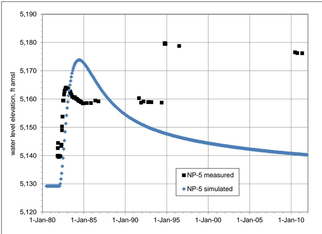
Figure 6.26. Measured and simulated water-level hydrographs in NP-5.
