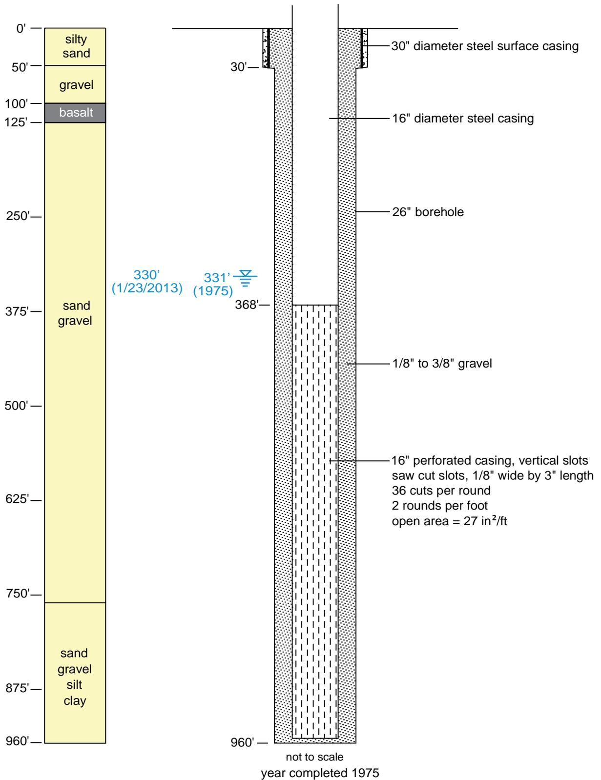
Figure B1. Well completion diagram for LRG-4652 (PW-1),
