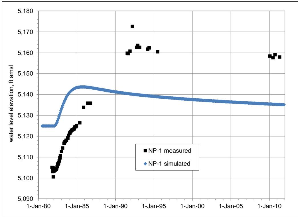
Figure 6.22. Measured and simulated water-level hydrographs in NP-1.
