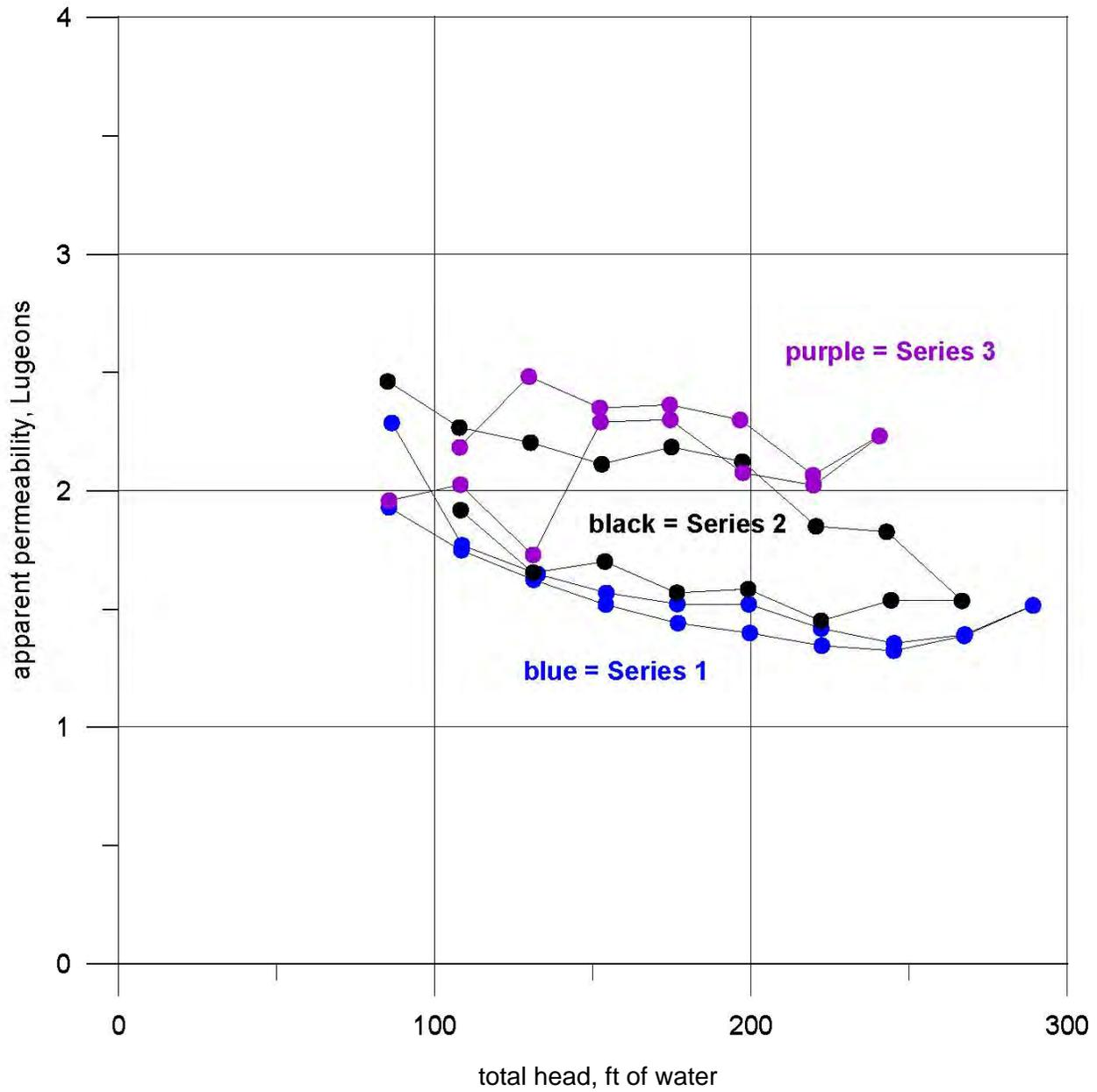
Figure 11. Apparent permeability from pressure injection test, New Mexico Copper GWQ 11-25, Zone 2 (150-197.7 ft), Series 1, 2, and 3, August 16, 2011.
