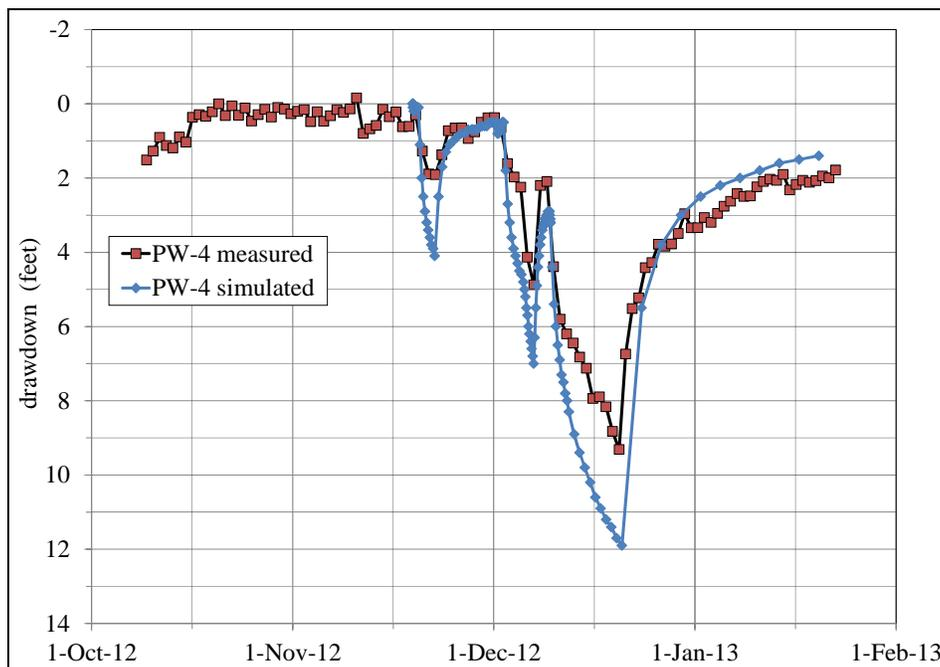
Figure 6.34. Measured and simulated water-level hydrographs in PW-4.
