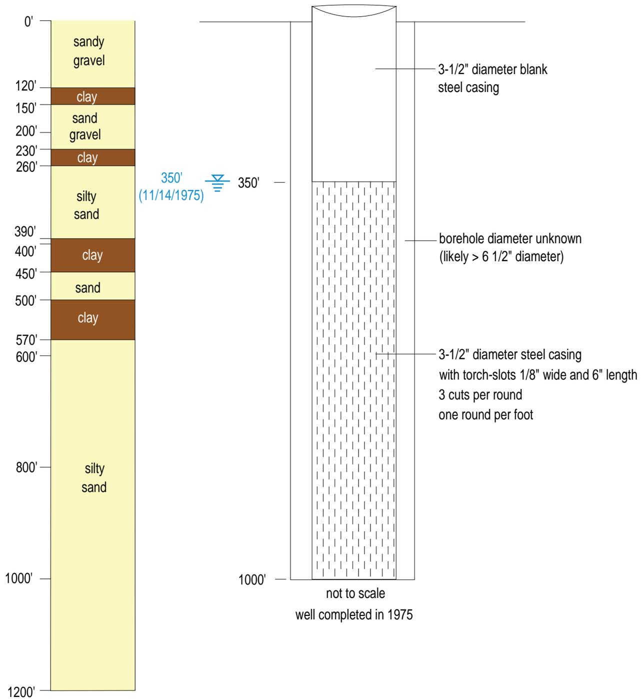
Figure B12. Well completion diagram for LRG-4652-S-11 (MW-1), Copper Flat Mine, Sierra County, New Mexico.
