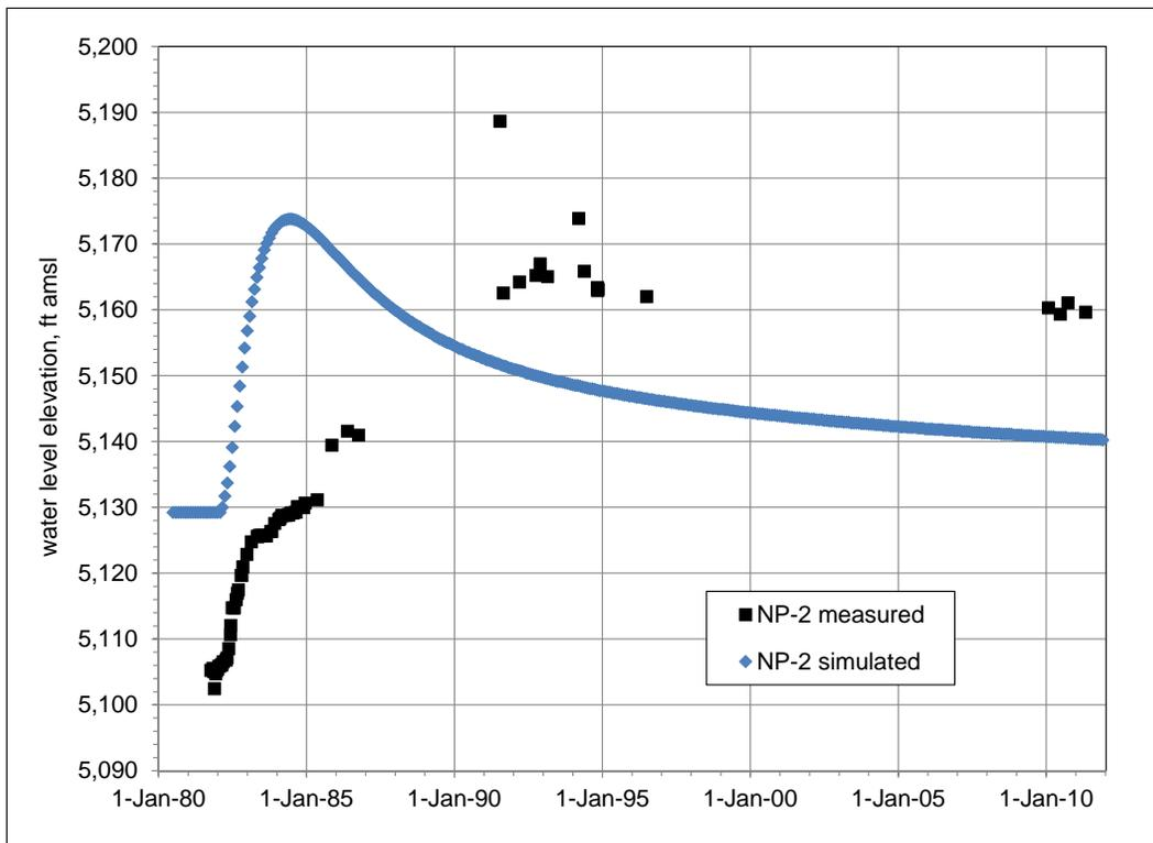
Figure 6.23. Measured and simulated water-level hydrographs in NP-2.
