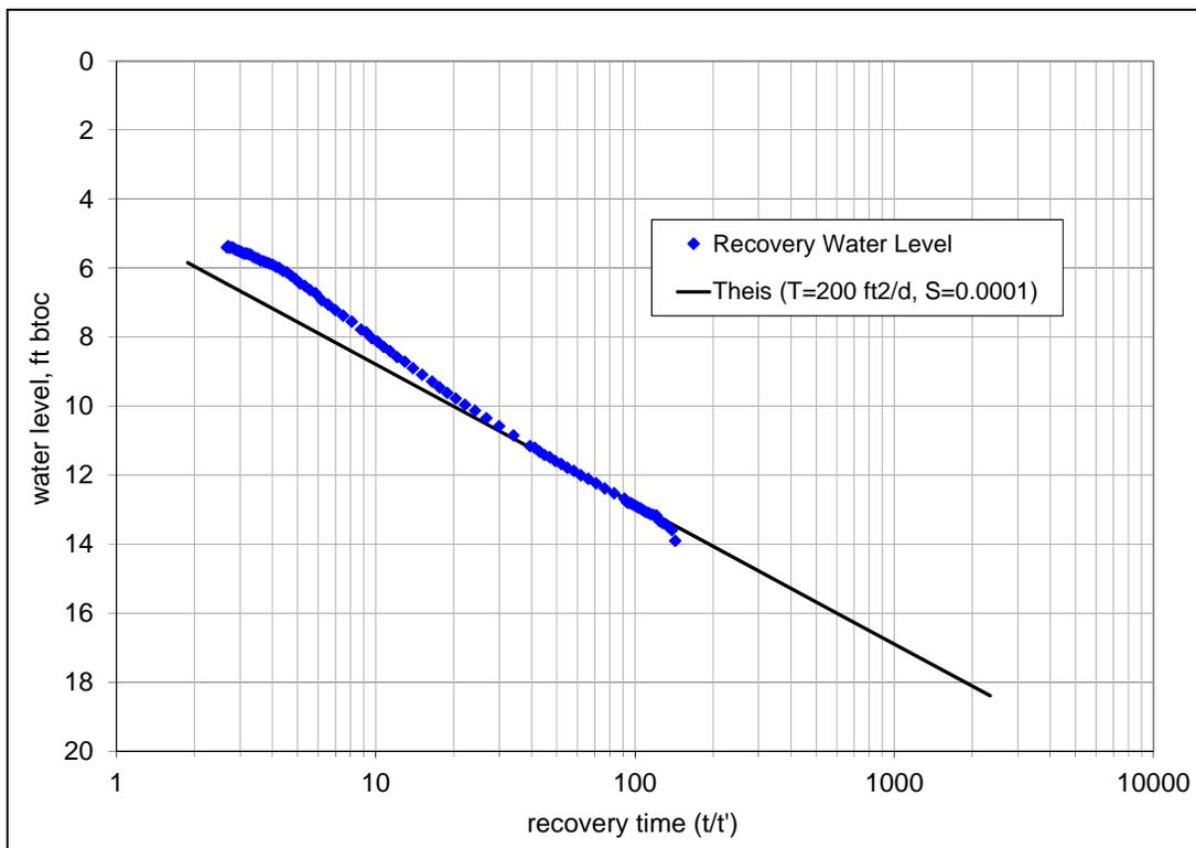
Figure 5.20. Recovery in GWQ-17 after 1994 pumping test.
