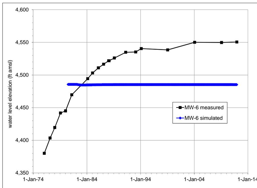
Figure 6.14. Measured and simulated water-level hydrographs in MW-6.
