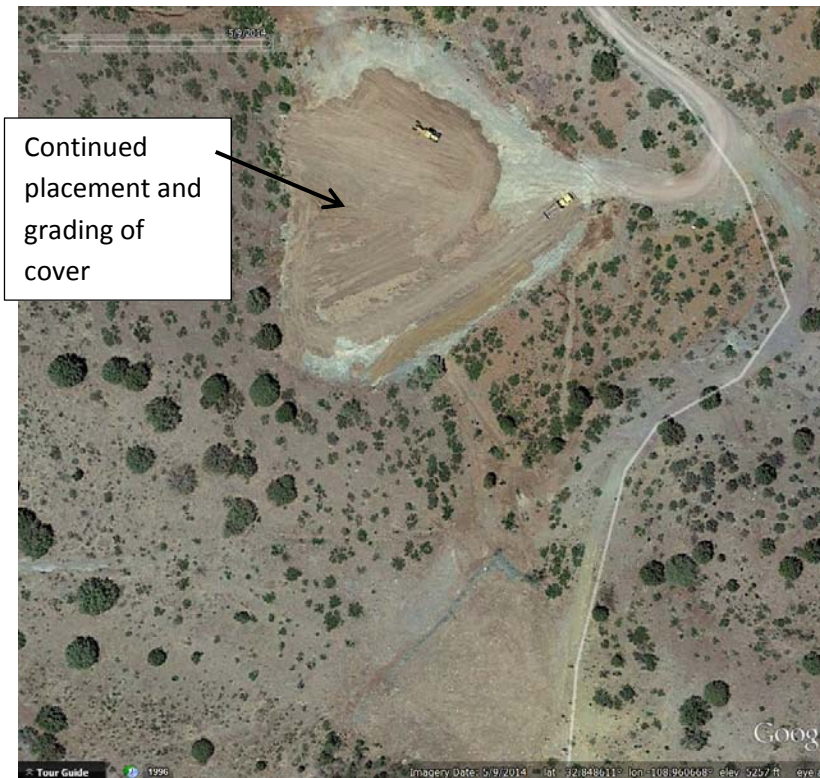
Figure 4: Center Mine Aerial Photograph from May 2014. Continued placement and spreading of cover soil over the regraded stockpile area.
