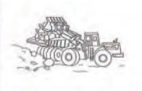
The Loading and Hauling of Rock System balances the productivity of loading equipment to hauling equipment. It is assumed that the hauling equipment will encounter light traffic and will move up no considerable grades on the haul route. The Expanded System Listing shows Loading and Hauling systems that use either a track or wheel front-end loader Track loaders indicated range from 1-Cubic Yards capacity to 4-1/2 Cubic Yards capacity. Wheel loaders range from
