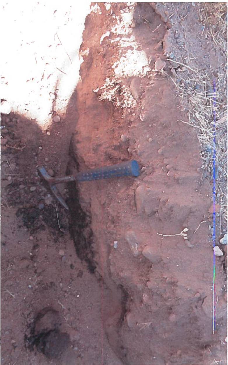
3. Backhoe trench along the west side of the site with manganese tailing showing at a depth of 12 inches. (February 9, 2018)
