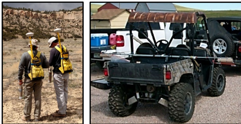
Figure 8: Example detector mounting configurations for walkover and UTV gamma scanning systems.
