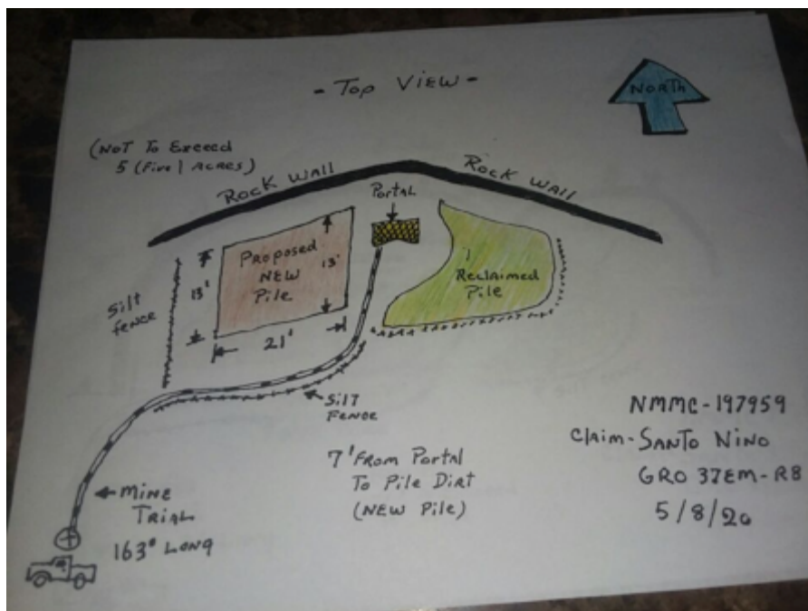
Exhibit B. Drawing Dimensions of New Pile, Reclaimed Pile, Mine Trail, Portal and Rock Wall
