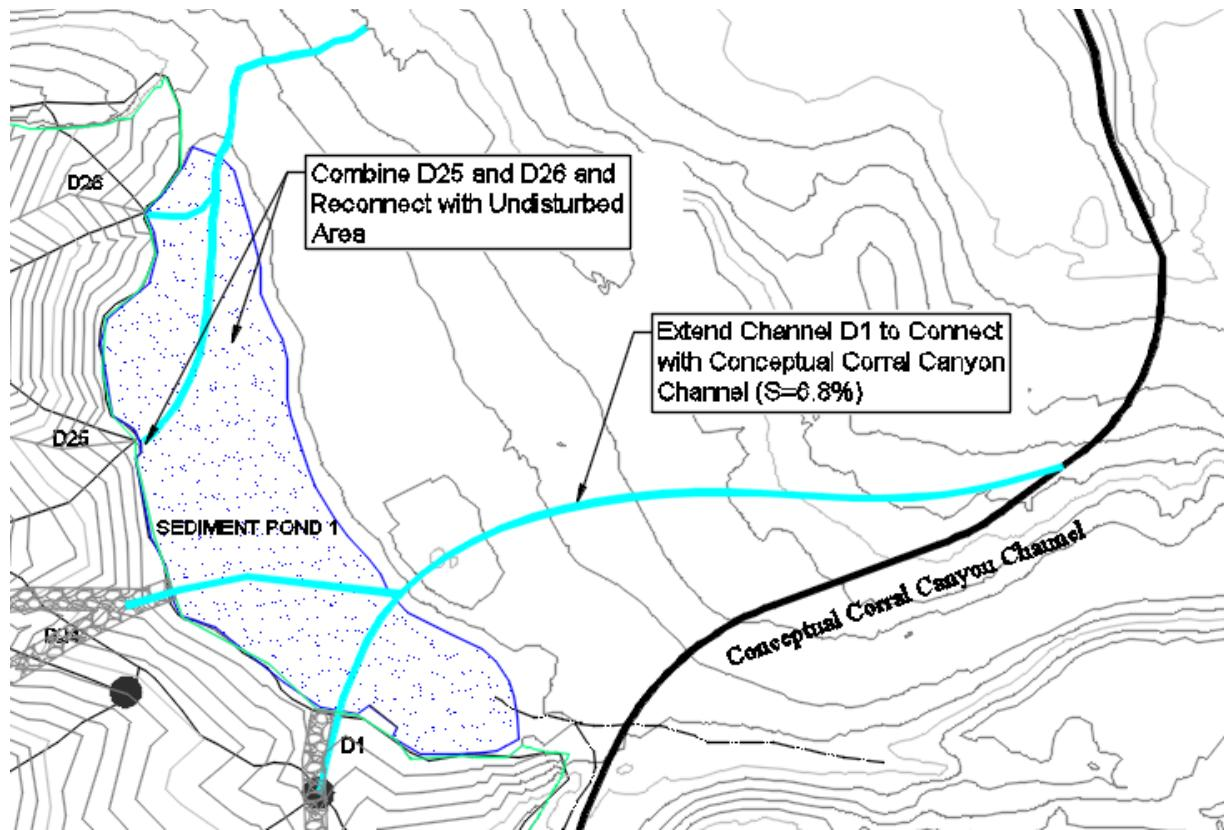
Figure 1. Conceptual Channel D1 Alignment that Flows into Corral Canyon at Mine Closeout
