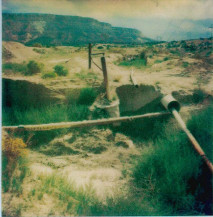
a) Discharge point from slimes pond. Discharge travels southward under road finally joining Sec. 35-36 pond system final discharge.
