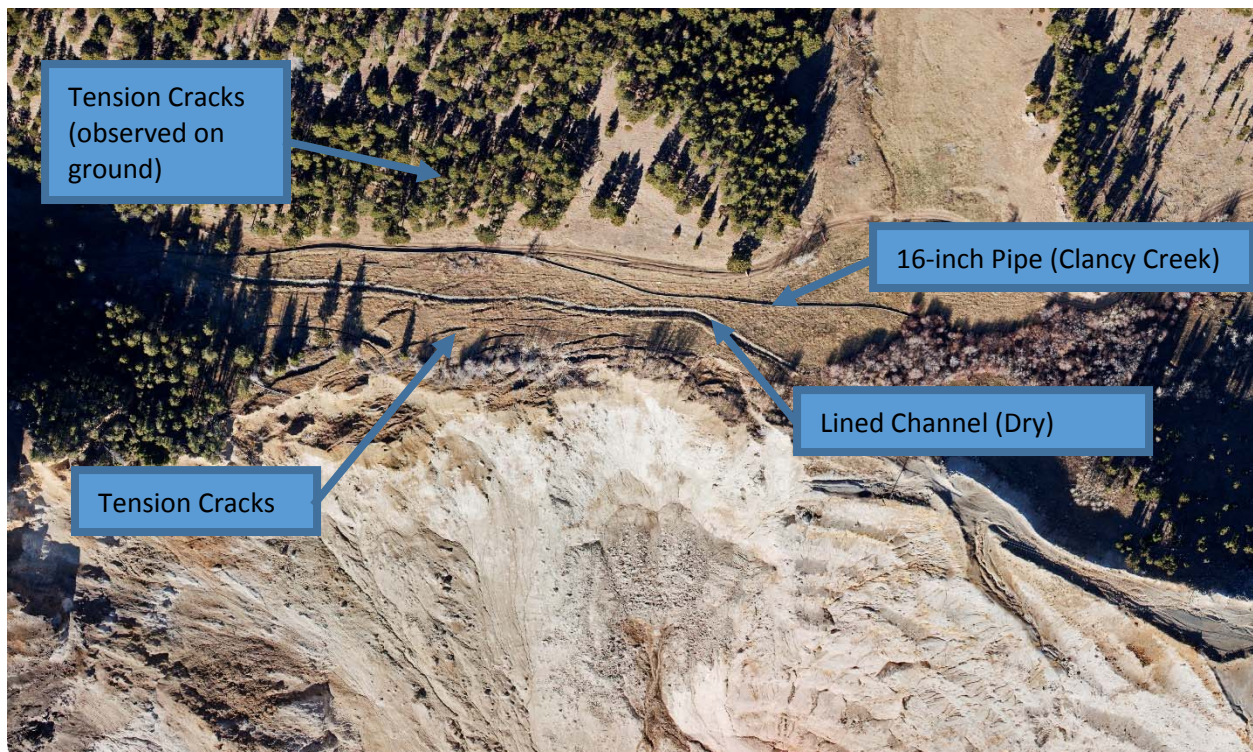
Figure 5. Montana Tunnels Open Pit Highwall Failure Along Clancy Creek. (Photo by Christopher Boyer)
