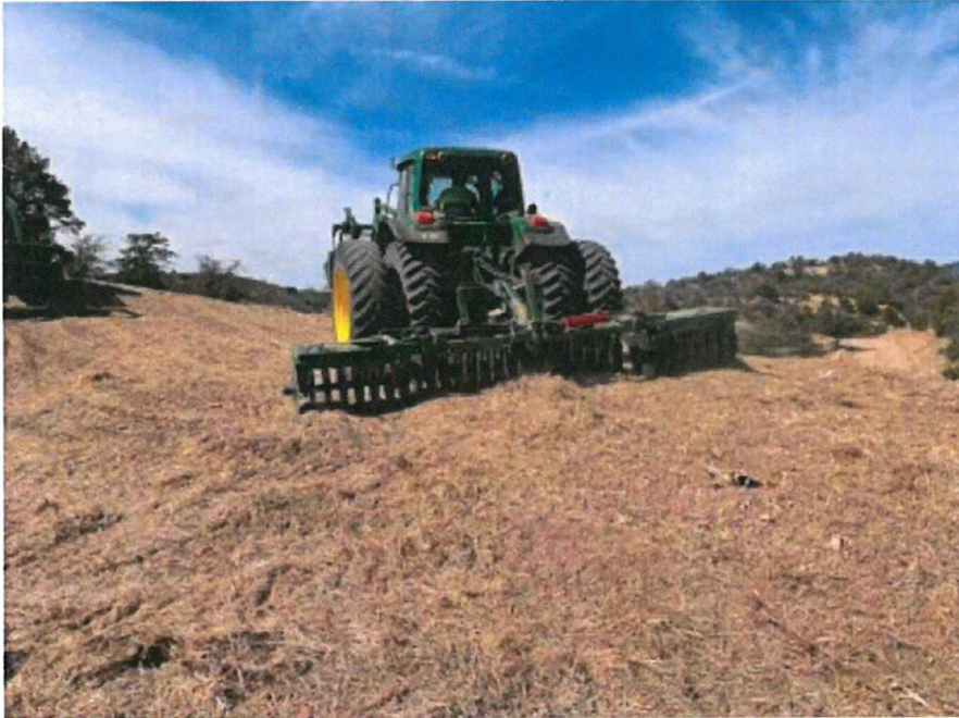
Figure 1. Crimping mulch after seeding (June 2022)
