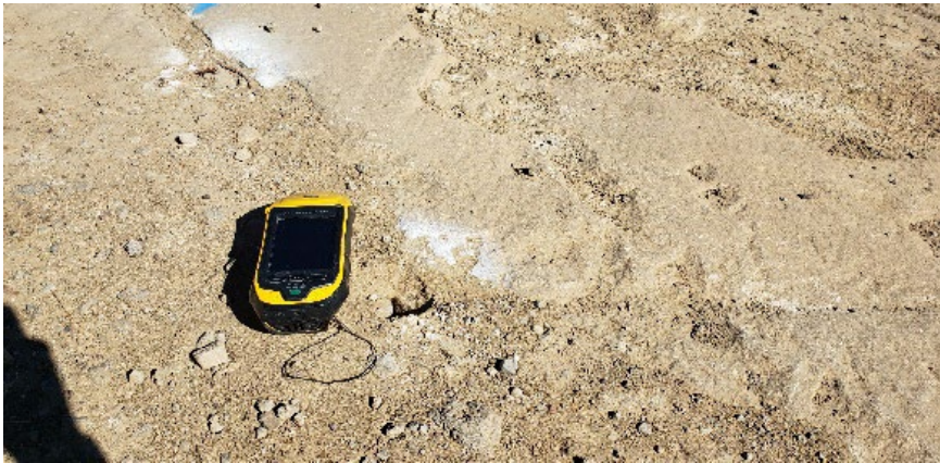
Photo 11. Logging subsidence features in County Road A-25 with GPS unit.
