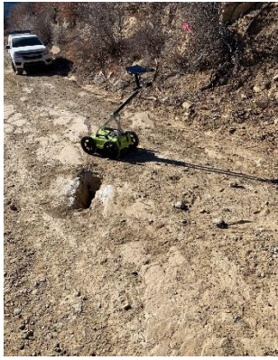
Site photo of the crack in the rocky area being scanned.
