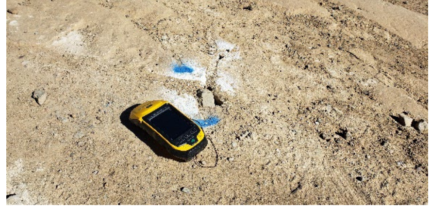
Photo 10. Logging subsidence features in County Road A-25 with GPS unit.
