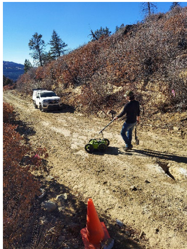
Photo 3. GPRS employee performing ground penetrating radar (GPR) inspection.
