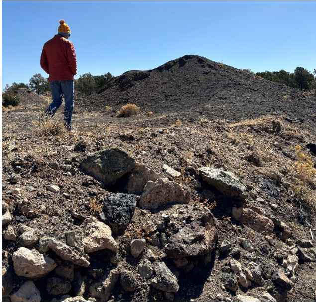
FIGURE 35 ORE PILE WITH MATERIAL COMING DOWN INTO DRAINAGE
