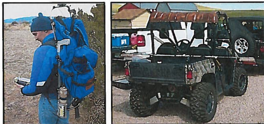
Figure 5: Example detector mounting configurations for backpack and ATV gamma scanning systems.
