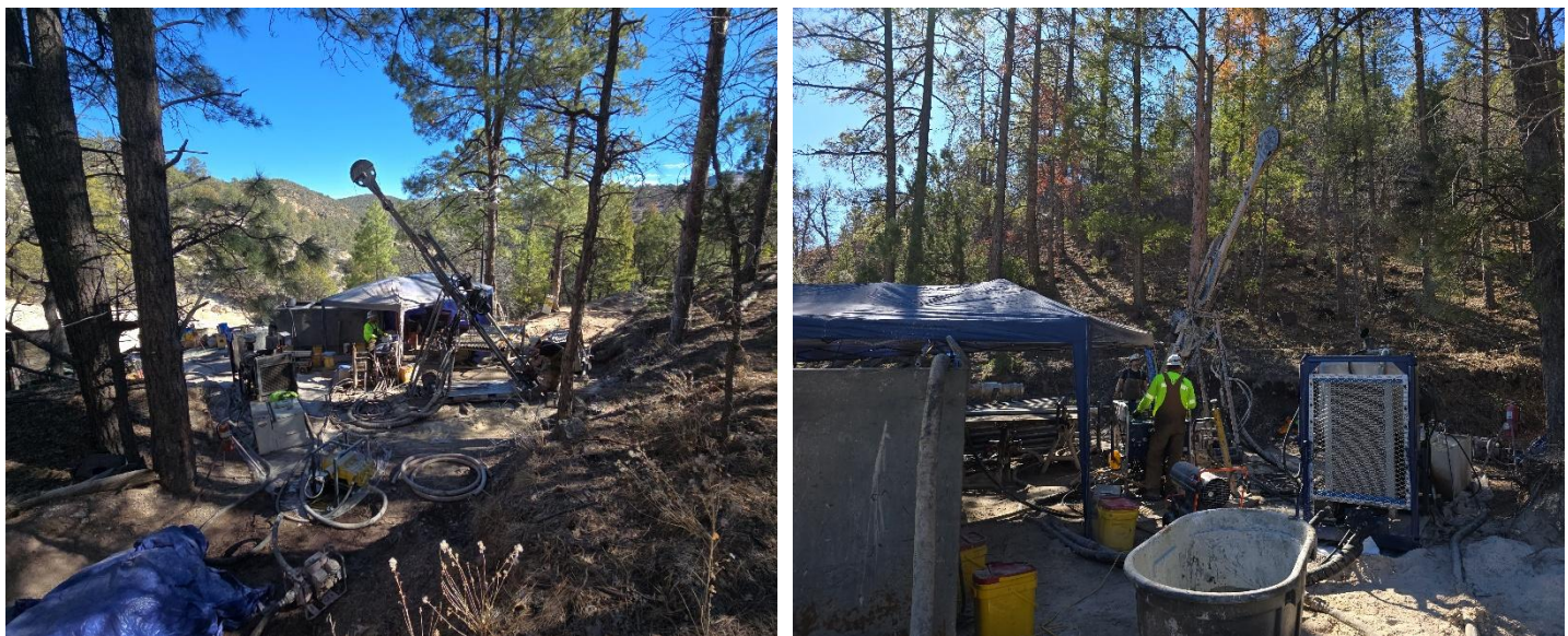
Figure 1 – Images from 2026 operations conducted under Summa’s MMD Part 3 Permit at site DP04 depicting typical skid-mounted core drilling activities.
