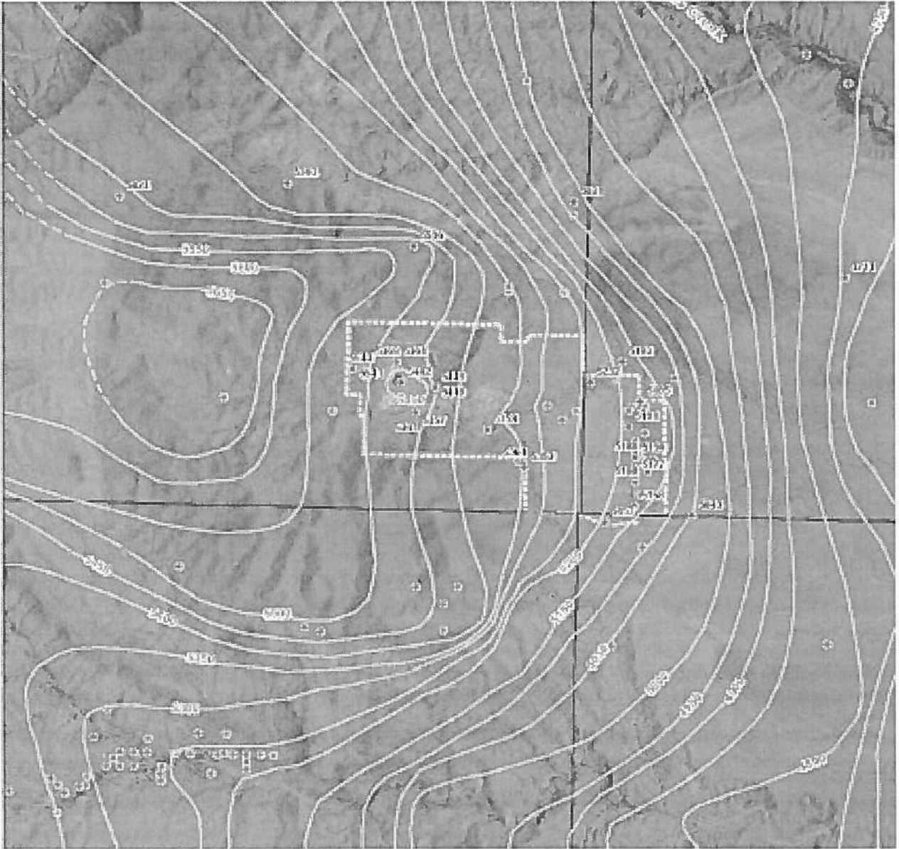
Figure 2: Potentiometric surface around the mine site in 2011 (Source: Figure 5.1 from Jones et al (2014)). The closed contour around the mine pit is 5450 feet above mean sea level.
