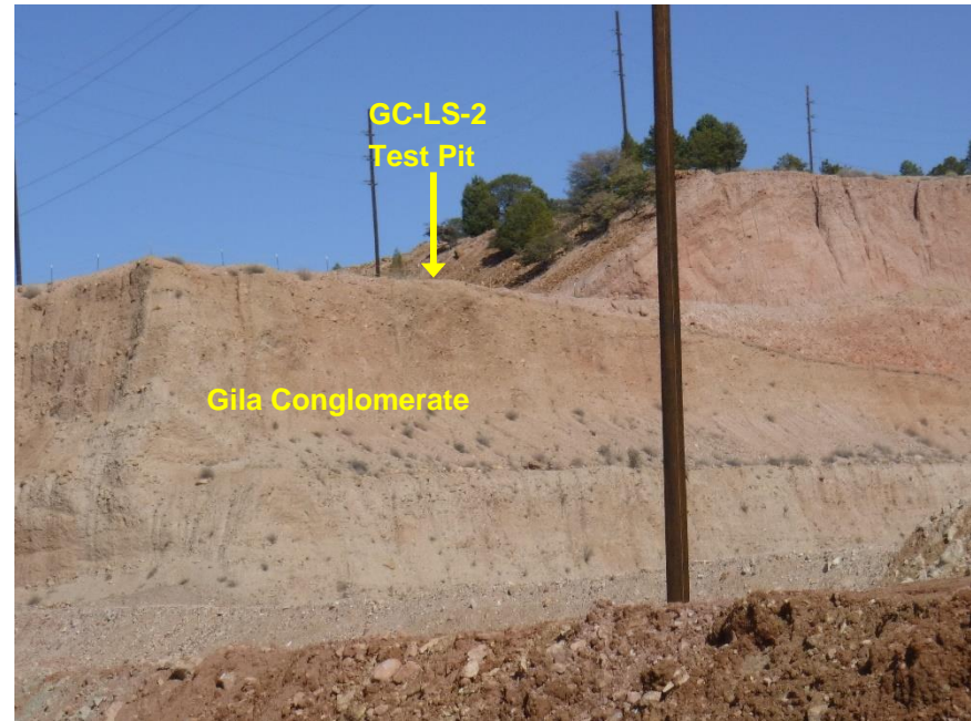
Photo B: Test pit GC-LS-2 location from below showing reddish waste rock from the Savanna Pit overlying GCRCM
