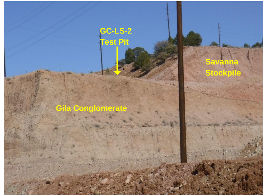
Photo B: Test pit GC-LS-2 location from below showing reddish waste rock from the Savanna Stockpile overlying GCRCM
