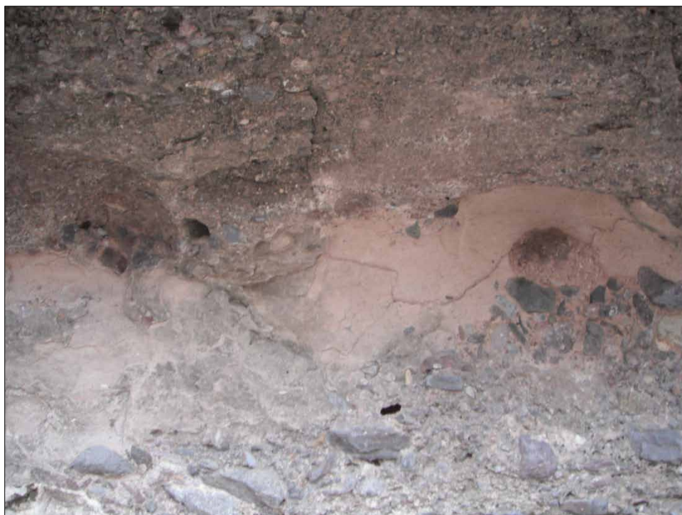
No. 56 – Close up of clay lenses and cemented gravels in the north wall.
