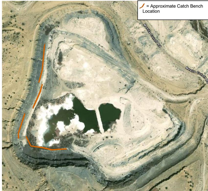
Figure 13: Simulated Rockfall Bench Cleaning Locations
