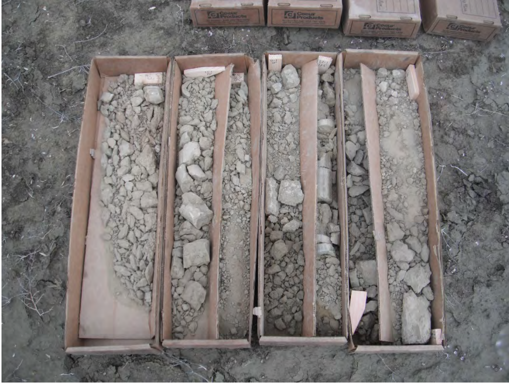
Photograph 11. L1-1 (all cores): 0' (bottom left) to 20' (top right) bgs
