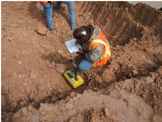
Measuring in-situ density – 5B Lysimeter
