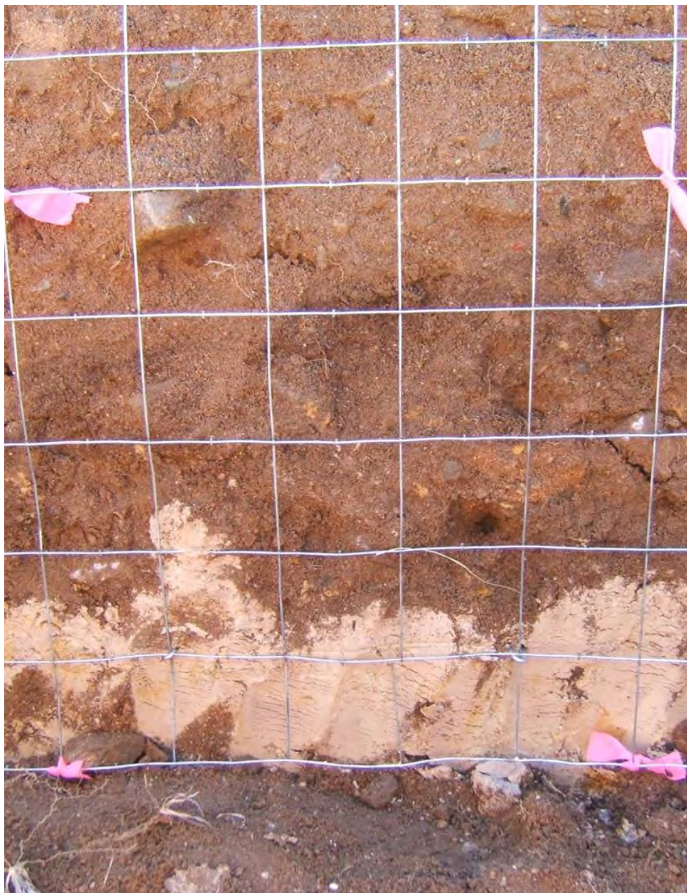
FIGURE 12 TONGUING OF TAILING IN THE BASAL CONTACT ZONE OF THE SOIL COVER. WIRE MESH GRID SPACING IS 10 CM.
