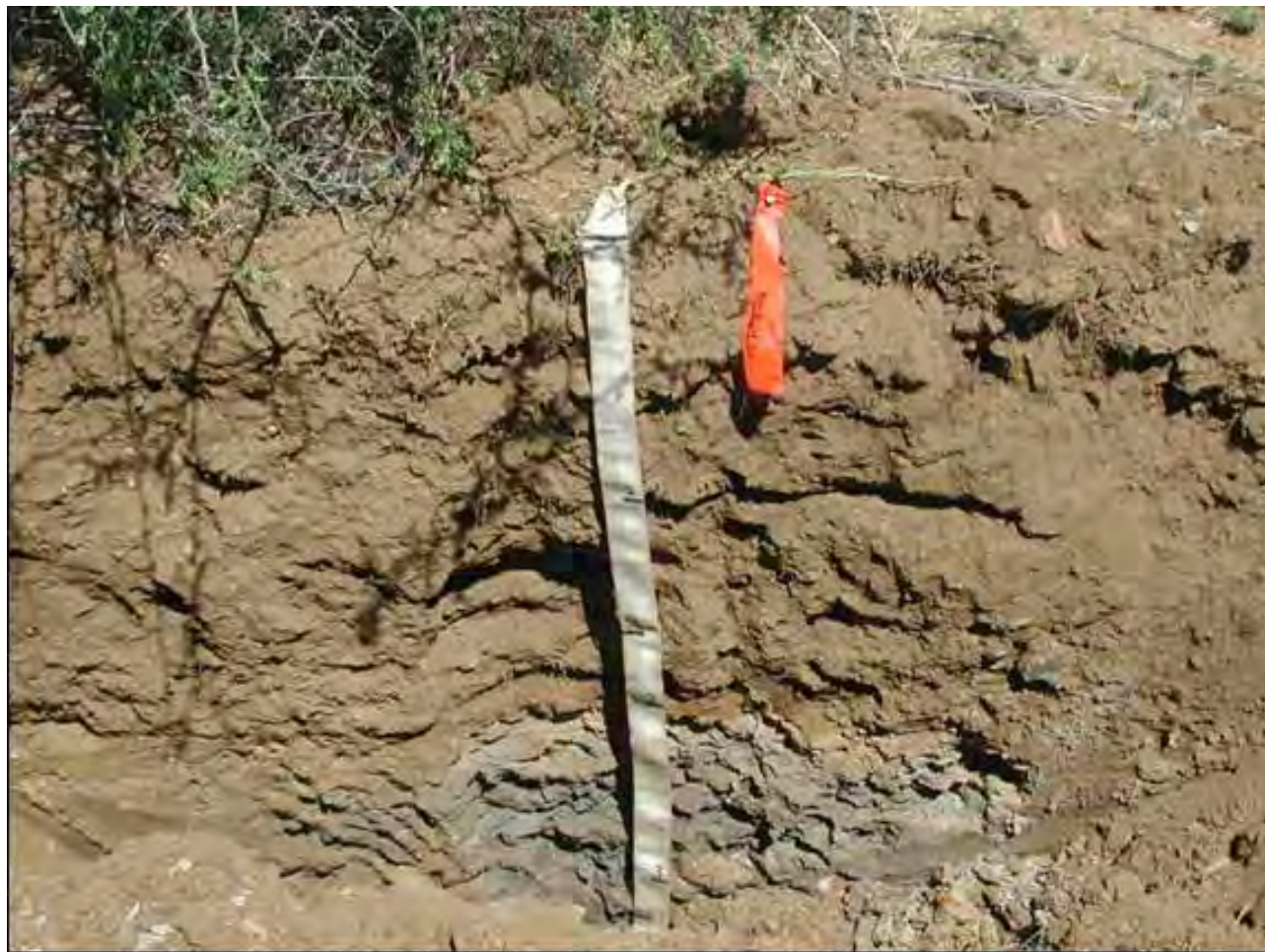
FIGURE 11 COVER SOIL OVER TAILING AT SITE TRT-1. THE TAILING IS EXPOSED IN THE PIT WALL AT APPROXIMATELY 60 CM BELOW GROUND SURFACE.
