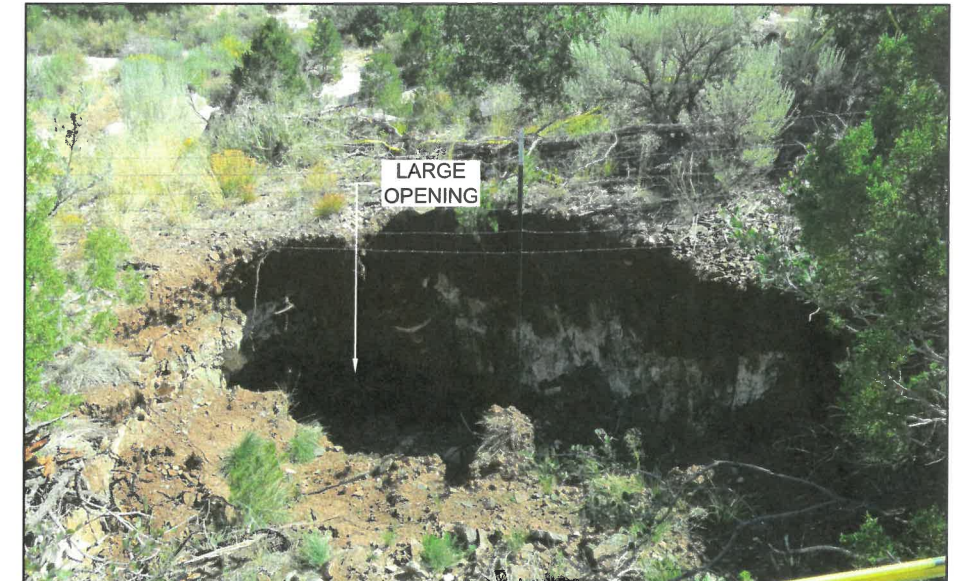
3 SUB-1 OPEN STOPE - EXISTING CONDITIONS 8 LOOKING EAST TOWARDS LARGE OPENING AND HIGHWALL
