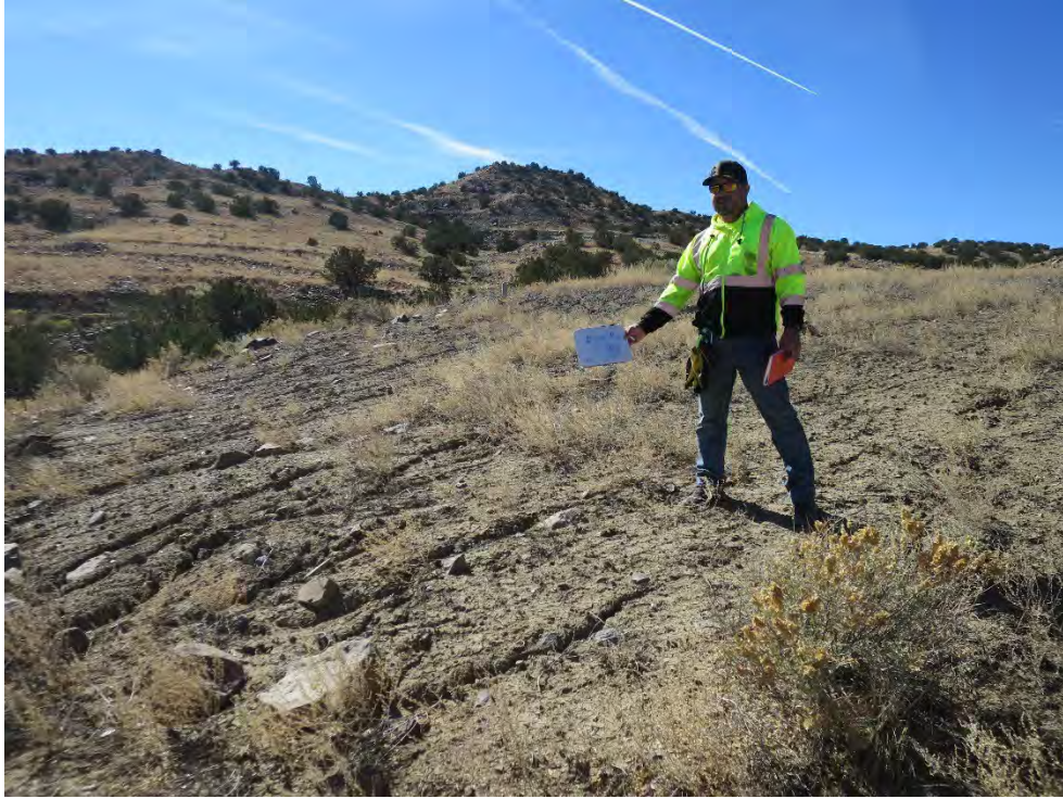
Photograph 23 - (VS-10 Photo Area E, looking south): Interrilling along gentle sloped area.
