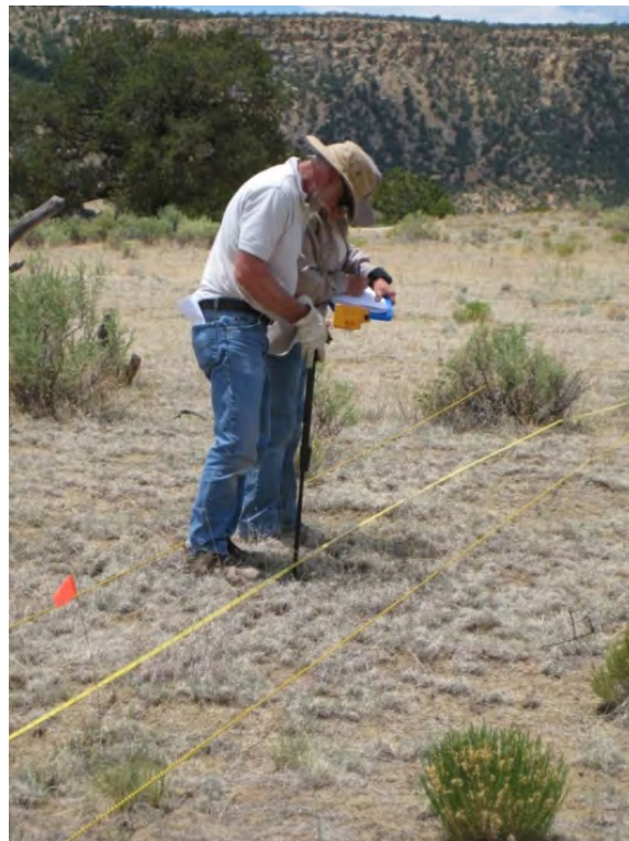
Figure 1. Use of an optical laser device to measure cover.
