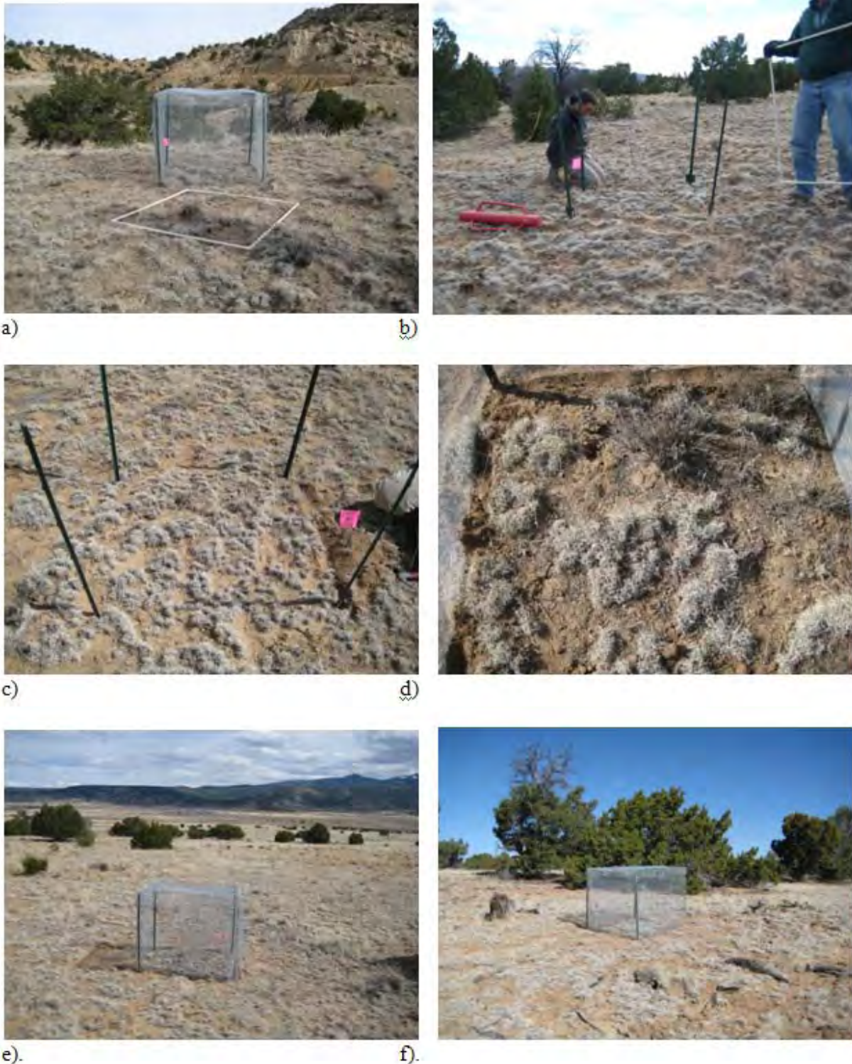
Figure 4. Enclosures that were erected at the project site. (a) A completed enclosure and the template frame. The 1 m x 1m frame in the foreground was used as the template for erecting the four support rebars (one at each corner) shown in (b). A narrow trench was dug so the sides of the enclosure were buried (c) and then the trench completely filled in with the soil that was removed so that erosion would be avoided (d). Completed enclosures with "lids" secured by baling wire are shown in (e) and (f).
