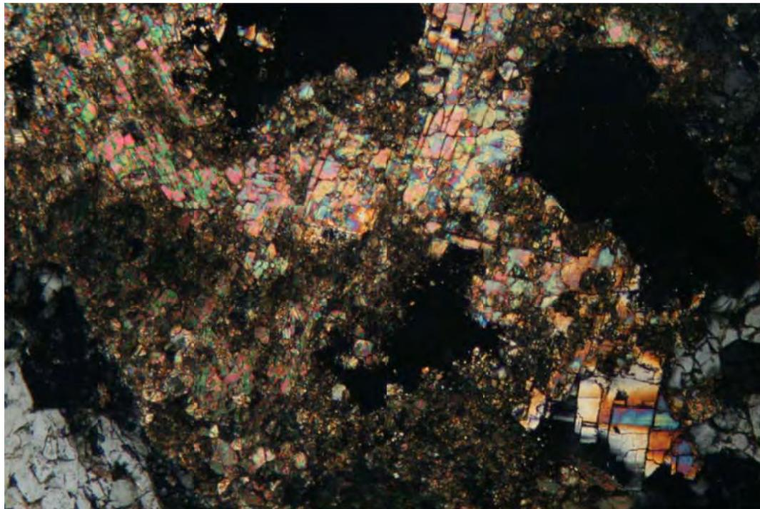
**Figure 14-1: Carbonate mineral within quartz matrix. (XPL at x 10 magnification.
