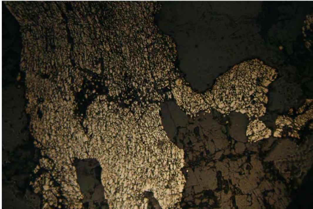
**Figure 14-2: Pyrite within quartz matrix. (reflected light at x 10 magnification.
