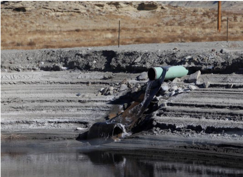
Water pumped from the San Juan Mine flows from a sedimentation basin into a pond, Thursday, Nov. 14, 2019. The water is mainly the result of spraying along the underground mine to reduce dust levels, according to Dan Mumm, environmental engineer at the mine. (Photo: Hannah Grover/The Daily Times)
