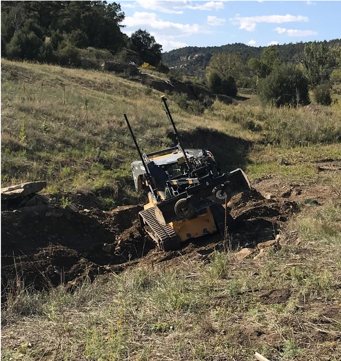
Figure 6. A John Deere track loader equipped with Level Best attachment and Topcon 3D-MC grade control software
