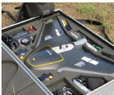
Figure 1: The Trimble UX-A Aerial Imaging Rover used in areal mapping.
