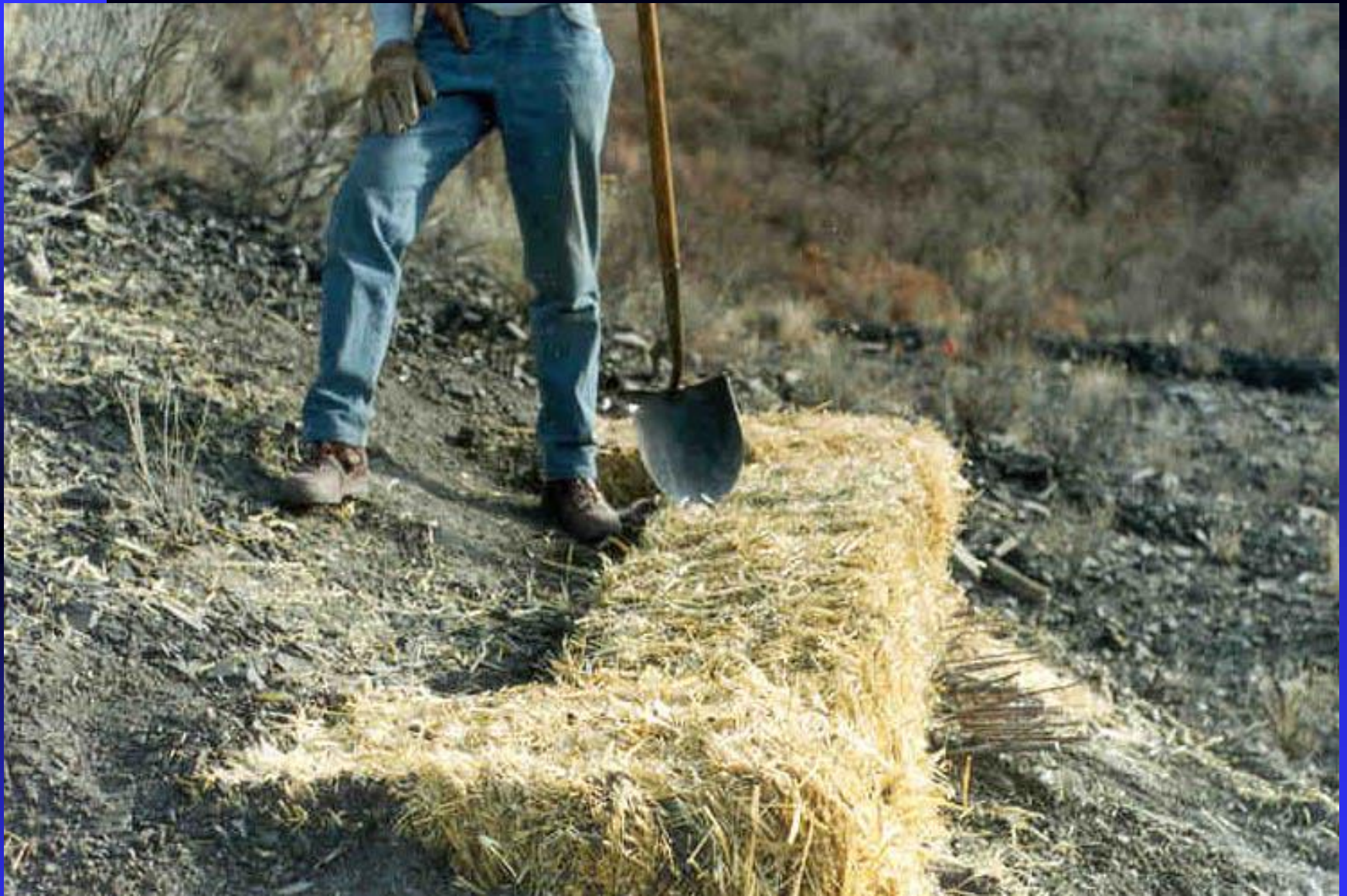
Straw bale terrace test installation
