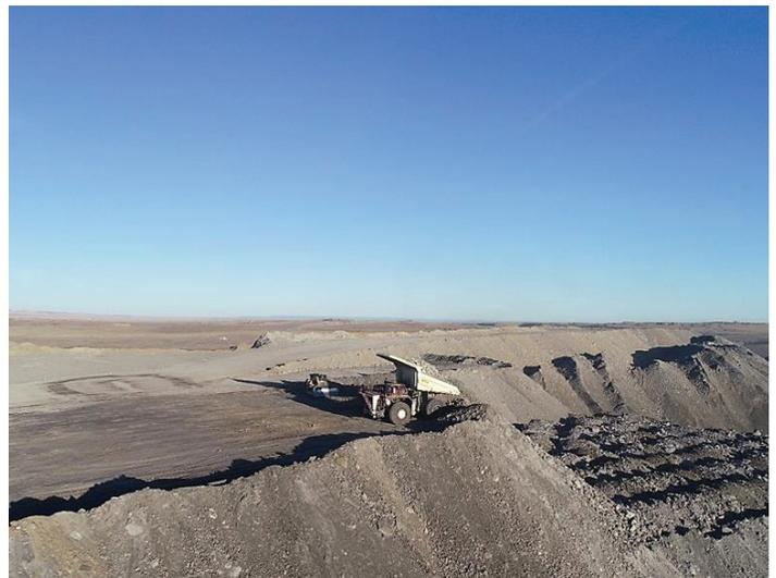
*At Peabody's El Segundo Mine, a "shovel and truck" operation to move material prior to a dozer grading the site to the landform design*
