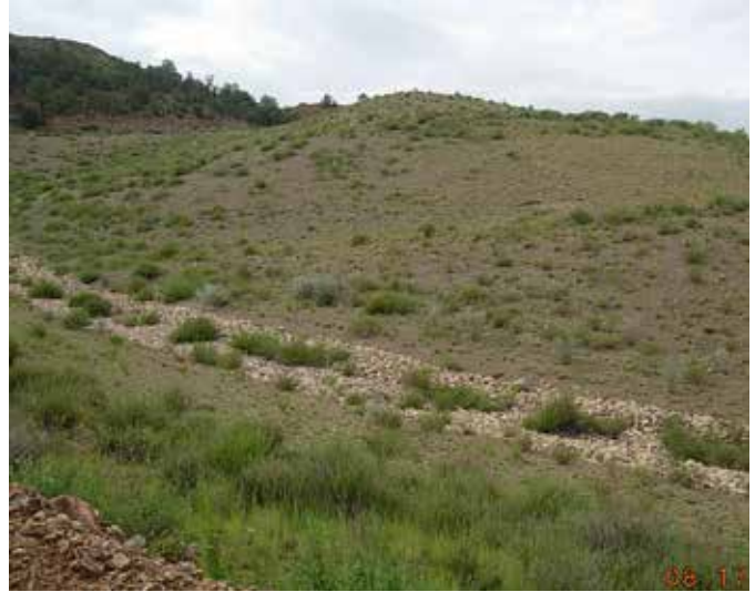
Test plots to test Little Rock Precambrian granite cover material at Tyrone Mine, 2022
