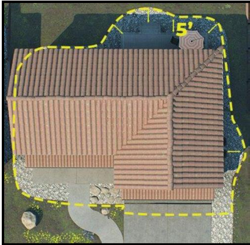
Figure 12. The area for a five-foot non-combustible buffer around a home (Courtesy of Wildfire Prepared, a Program of IBHS).
