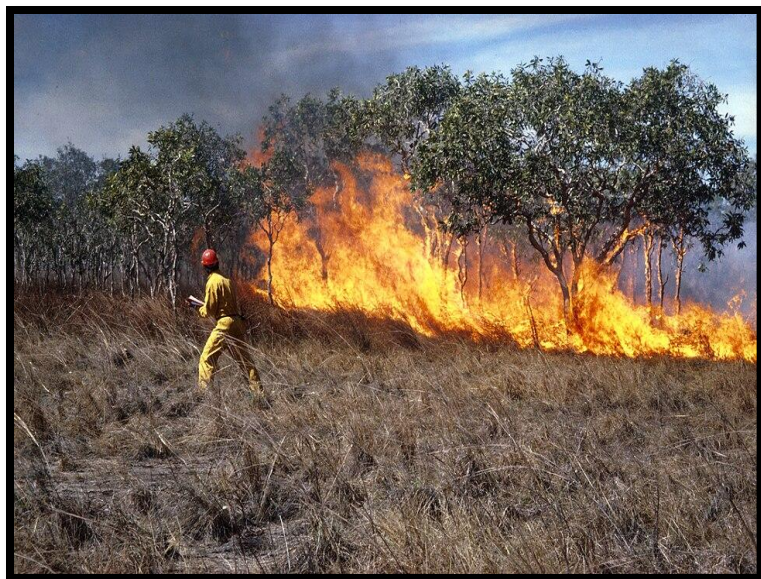
Figure 19. Example of a grassfire experiment. Note the increase of flame length in the transition from grass to trees, which expresses the change from a ground fire into a crown fire (Courtesy of https://commons.wikimedia.org/wiki/File:CSIRO_ScienceImage_558_Grassfire_Experiment.jpg ).
