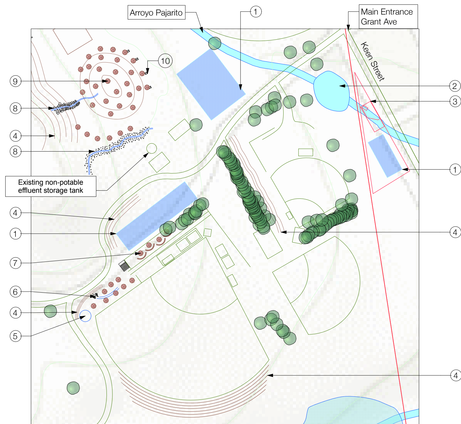
Figure 24c: Suggested green stormwater infrastructure designs.
