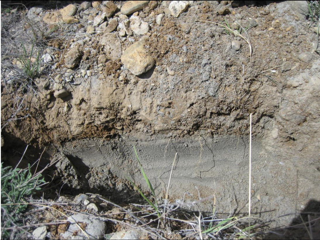
Photo 3: Soil/tailing sampling location – cover (brown soils) and tailing (gray material)
