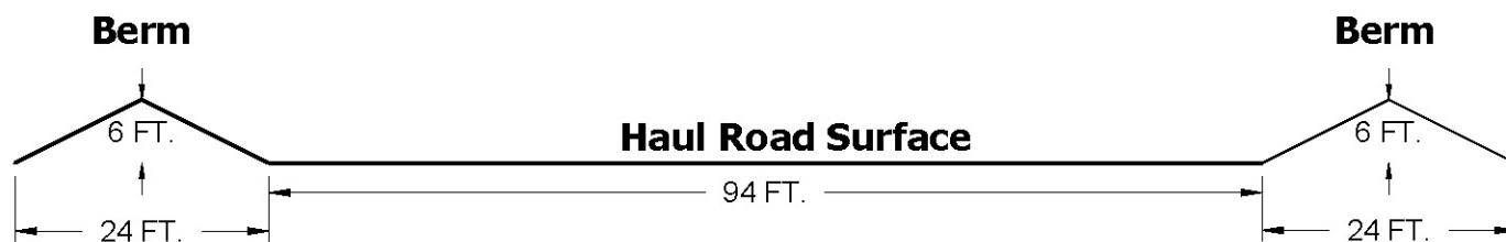
Typical Haul Road Cross Section Dual Berm
