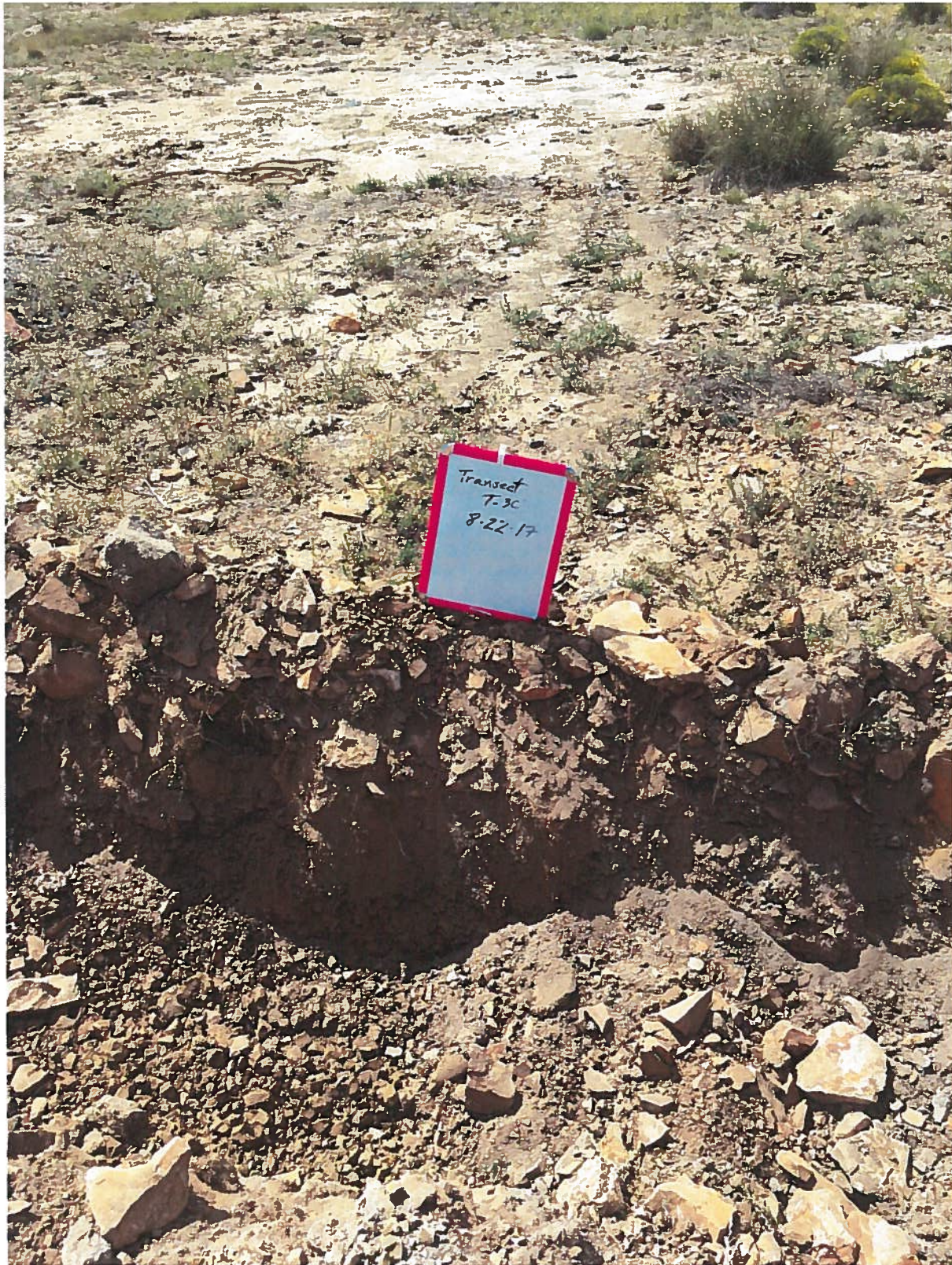
Figure 17. Photo: QLUH0714. Trench T-3C on east side of waste pile. Note blocky and angular lakebed clays as well as fragments of sandstone rock with yellowish chroma (limonite).
