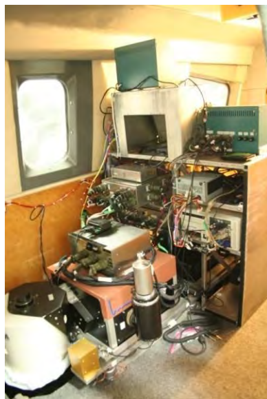
Image 14: View of chemical sensors: high speed infrared spectrometer, lower left corner; infrared line scanner is out of view behind the line scanner.
