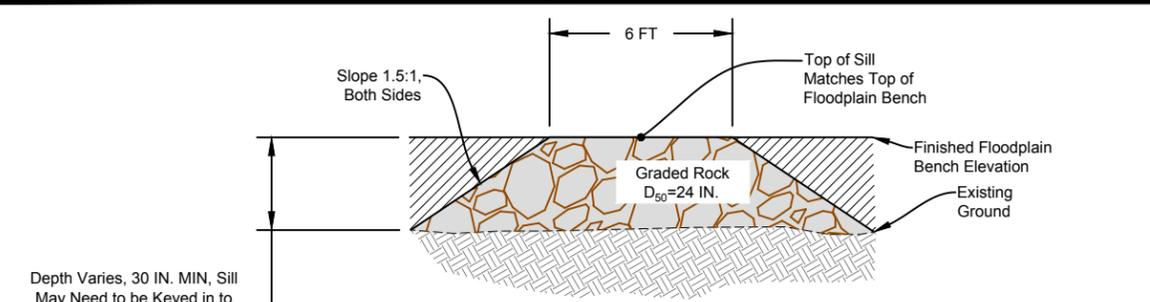
**S04** Typical Graded Rock Sill Section
