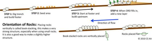
**Orientation of Rocks:** Placing rocks vertically is called book-stacking, this makes a very strong structure, especially when using small rocks. It is also a good way to make a slightly higher structure.
