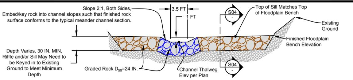
**S03** Typical Graded Rock Riffle & Sill Section
